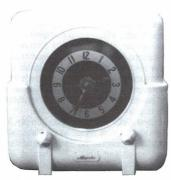
MAJESTIC MODEL 5-T — The semi-circular dial of this 1940 Art Deco set is behind the upper half of the outer silver-colored ring of the glass clock face, and appears only when the pilot light shines on it. The sole function of the line cord resistor is to drop the 117 VAC to six volts for the pilot light. Though this could be called a clock/radio, the clock operates independently of the radio and will not turn your coffee on in the morning. (David Kraeuter - Washington, PA)
