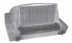
PHILCO MODEL 53-566 – This odd-shaped 1953 table model covers AM 550 to 1600 Kc on the broadcast band. Note the wording "Special Services" and the pictures of a phone, ship and airplane on the slide rule dial. (Doyle Roberts – Clinton, AR)
