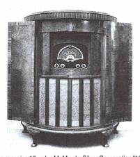
The massive 15-valve McMurdo-Silver Corporation "15-17", ca. 1938. This 15-valve console, made in England but of American design, was introduced to England in 1937 by McMurdo. Six wavebands cover 4 to 2200 meters. The whole chassis is chromium-plated and is housed in a solidly built, semicircular, 4'x 3'x 1'9" walnut cabinet, which also includes a 17" speaker and a record turntable.
