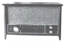
ZENITH MODEL T2542 — A 1965 AM/FM table radio with chassis 7M07, this set has an all-wood cabinet which is styled to match the television sets Zenith made that year. The 6-inch cone speaker and 3-inch electrostatic tweeter give the set a wider range of tone than most table radios. (Daniel Schoo – De Kalb, IL)
