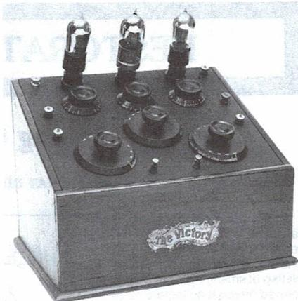
"The Victory," a 3-valve sloping panel receiver made from a kit in England in 1923.
