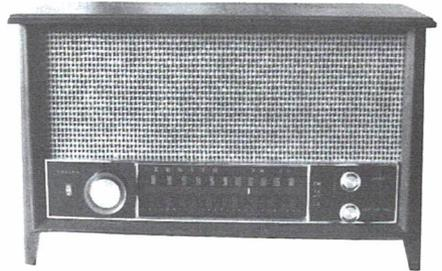
**ZENITH MODEL T2542** – A 1965 AM/FM table radio with chassis 7M07, this set has an all-wood cabinet which is styled to match the television sets Zenith made that year. The 6-inch cone speaker and 3-inch electrostatic tweeter give the set a wider range of tone than most table radios. (*Daniel Schoo - De Kalb, IL*)
