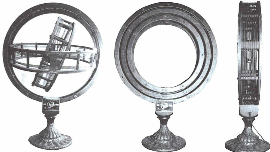
The Pratt loop is shown (left) expanded, (center) folded shut, and (right) folded shut from a side view.
