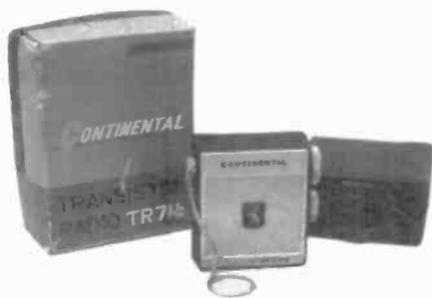
**CONTINENTAL MINI-TRANSISTOR RADIO** – This 7-transistor model uses a penlight battery and measures 2 1/2" by 2 1/2" by 1" deep. It has a brushed aluminum face, a key chain, and a vinyl carrying case. (Randy King – Lincoln, NE)
