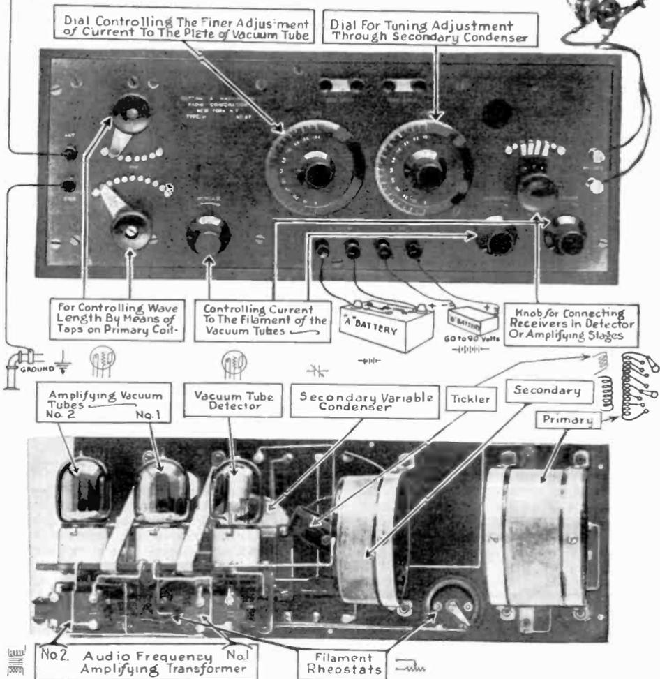
choked, so that control of the feed-back is provided by rotating the tickler coil. In one position, it is in line with the primary and secondary coils and gets the full strength of the induction. As it is turned from this position, the effect of induction is decreased so that the feed-back is gradually cut down.
