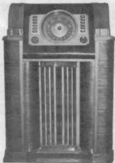
**CROSLY MODEL 03CB** – This large 10-tube floor model, circa 1940, with a waterfall front and a 12-inch speaker, has six push-button station settings and six push-button tone control positions, as well as 2 shortwave bands and a broadcast band. (Randy King – Lincoln, NE)
