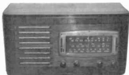
**FARNSWORTH MODEL BT1010** – This imposing 10-tube AC set from the late 1940s has two push-pull Type 6V6 output tubes and an 8-inch dynamic speaker. Note the unusual slider-type bass and treble vertical tune controls on either side of the dial escutcheon. (Gregory E. Jones – Westerly, RI)
