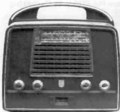
**PHILIPS PORTABLE MODEL LX444AB/03** – This early plastic foreign portable features SW/LW/MW, multivoltage or 67 ½-volt B battery and 1 ½-volt A battery. It has a bright pink case with a clear grille/faceplate and a swing-up metal loop antenna on the back, which has the same shape as the case. (*Randy King – Lincoln, NE*)
