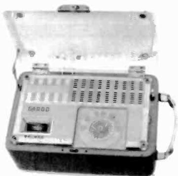
**GAROD MODEL 4A1** – This portable radio has a metal case, a molded plastic back and lid, a vinyl handle, and an antenna in the lid. It uses a 67 ½-volt B battery and a 1 ½-volt A battery. (*Randy King – Lincoln, NE*)
