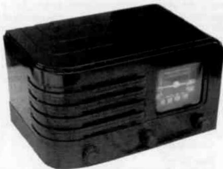
**STROMBERG-CARLSON MODEL 561** – This large Bakelite set was built in Canada in 1940 and seems uncommon in the States. It is an AC/DC superheterodyne, using six octal base tubes. The original set belonged to my family in the 1940s, but was lost over the years. Luckily, I found this identical set through a photo ad in A.R.C., which was also the source of the schematic from a Canadian reader. This radio was also produced as a battery farm set, Model 541. (*Ray Larson – W. Los Angeles, CA*)
