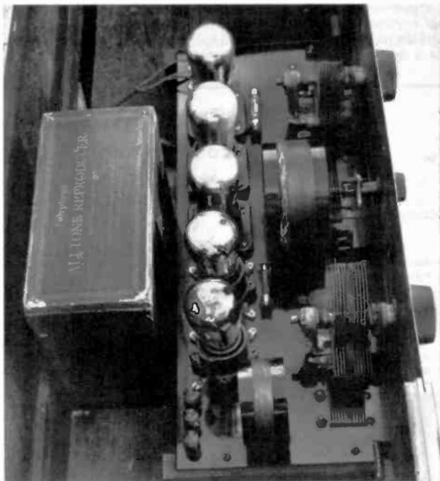
Figure 3. Inside view of the Orpheus showing the 5-tube chassis and the Alltone reproducer.
