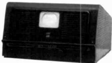
**PILOT MODEL TV-37** – This 1949 TV used 17 tubes with a 3-inch picture tube. At \$99.50, it was the first TV priced under \$100. (Tony DeMara – Mt. Clemens, MI)
