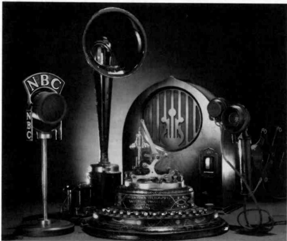
Figure 1. This Smithsonian press release photo includes an early NBC broadcasting microphone, a Magnavox R-1 horn speaker, an Edison stock telegraph printer (glass dome removed to eliminate glare), and a Western Electric telephone of the 1920s displayed around an Echophone Model S-3 cathedral radio. (Photo courtesy of Laurie Minor, Smithsonian Institution)
