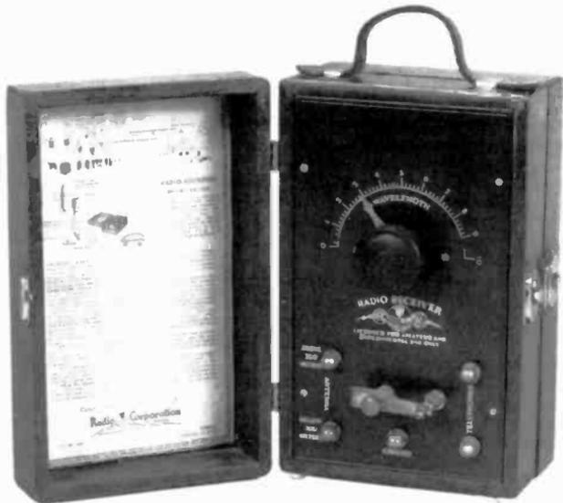
Figure 1. The Radiola I (Model ER753A), front or panel view.
