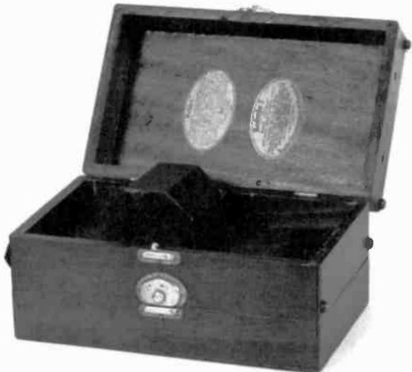
Figure 2. The Radiola I (Model ER753A), back or rear compartment view.
