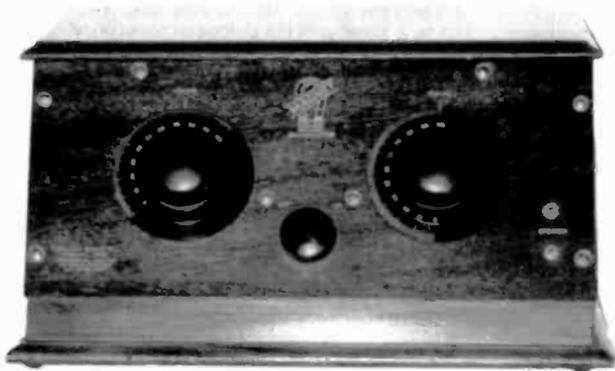
**CHELSEA RADIO COMPANY MODEL ZR-30** – This battery set, ca. 1925, is regenerative with a detector stage and 2 audio stages. A card inside the cabinet states that this set was made for Gimbel Brothers of New York. (George Hausske – Wheaton, IL)
