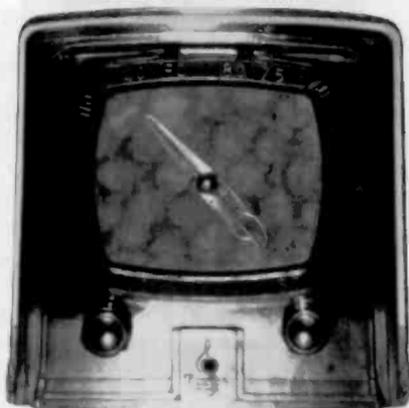
**EMERSON MODEL Q157** - This 4-tube AC/DC chassis would fit the rare Mickey Mouse radio cabinet. (George Hauske - Wheaton, IL)
