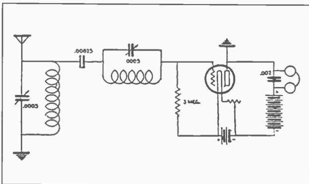
Figure 2. Schematic diagram of Sir Oliver Lodge's "N" circuit.
