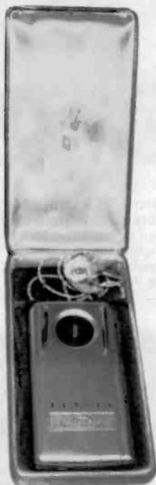
**ZENITH REGENT "PHONE MAGNET"** - This hearing aid, in its original box, uses 3 miniature tubes, an A battery and a 22½-volt B battery. The case is a shiny brass. (Howard Stone - Deer River, MN)
