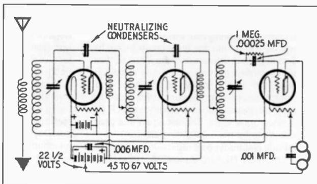
Figure 1. Schematic diagram of the Hazeltine Neutrodyne.
