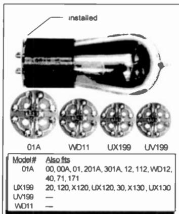
These tube repair wafers are solid-state devices for quick and easy repair of early vacuum tubes. The wafer is installed by simply sliding it over the tube pins and reinserting the tube into its socket. If the filament is intact, but there is little or no emission, the filament may be lit for best visual effect. However, the tube can be open filament.
