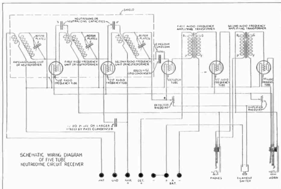
Figure 5. Schematic diagram of the Fada Neurodyne.
