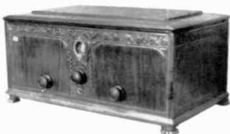
**KOLSTER MODEL K20** – This AC set, circa 1925, is in stark contrast to the earlier Kolster battery sets. This set contains no pot metal; it is all cast aluminum. Kolster must have recognized the deficiencies of the 6D-6K models and corrected them. (Walter V. Worth – Wollaston, MA)
