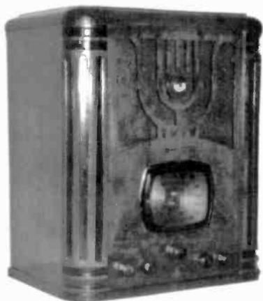
**EMERSON MODEL C134** – This large (21" high) tombstone has the Emerson "Gemlaid" dial, 5 control knobs, 8 tubes and an 8" speaker. Manufactured in 1936, this handsome 3-band radio is an excellent performer. Notice the magic eye located in the middle of the speaker grille. (*Wayne King – Shelbyville, KY*)
