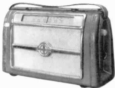
**DUCRETET-THOMSON MODEL TR854** – This circa 1962 transistor portable by the well known French company has 3 bands, AM/SW and LW, as is common in Europe. The case is built of molded plywood and covered in fine leatherette. (Walter V. Worth – Wollaston, MA)
