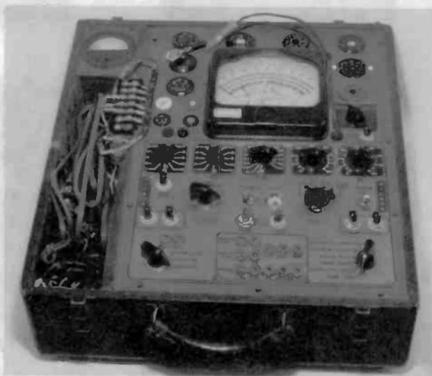
Figure 2. The Hickok 550X Dynamic Mutual Conductance Tester.
