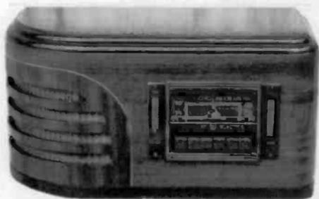
**GENERAL ELECTRIC MODEL HJ-624** - The rounded end and distinctive inlaid veneers make this 1939 set very attractive. It uses 7 tubes, one of which is a ballast tube. Although seemingly out of place in larger cabinets, its compact chassis was also used in console Model J-65 and others. (Spencer J. Doggett - Washington, MI)
