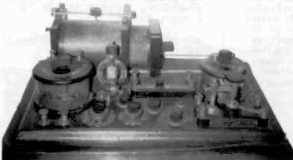
**WIRELESS RECEIVER** – Licensed by Wireless Specialty Apparatus for the Murdock Co., this crude receiver uses an Audion bulb. Pre-1920s receivers are not seen at flea markets very often. (*Joe M. Nocera – New Castle, PA*)
