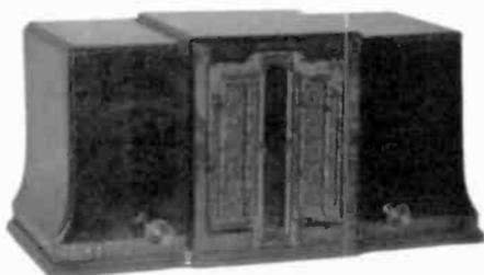
**HOWARD MODEL S** – Sold by the Howard Radio Company of South Haven, Michigan, this set with its unusual form has a classy look, featuring Deco styling and a vertical dial. The 8-tube (2-34s, 2-30s, 2-49s, 1-32, 1-1A6) standard broadcast receiver required 3 batteries (135V "B", 9V "C", 2V "A") circa 1934. (Wayne King – Shelbyville, KY)
