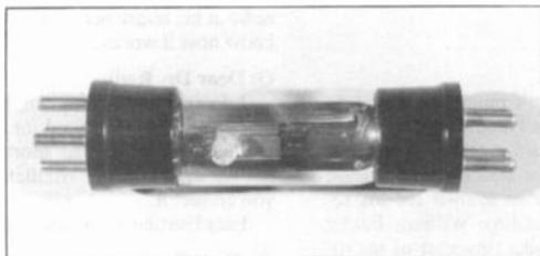
DUO-TUBE is a revolutionary double ended tube that has two filaments! If one filament loses emission or burns out simply reverse the tube and you're back in service!
