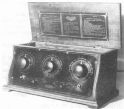
Figure 2. The "Kardonstrip," a TRF 5-tube set using riveted brass or bronze strips, which eliminated some wiring and soldering, ca. 1925.
