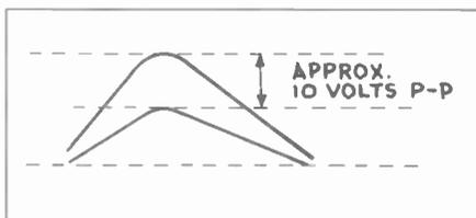
Figure 2. Oscilloscope waveform at 120 Hz sweep frequency.
