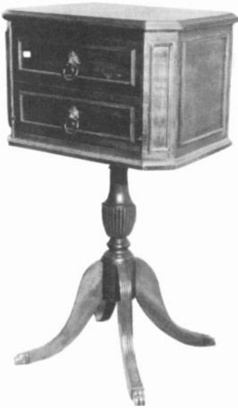
**WURLITZER MODEL 5U** – The two drawers in this Duncan Phyfe table pull down to expose the front of the radio — a style popular for only a few years around 1938. The cabinet of solid mahogany is very well built. The completely enclosed chassis has 5 tubes. *(Walter V. Worth – Wollaston, MA)*
