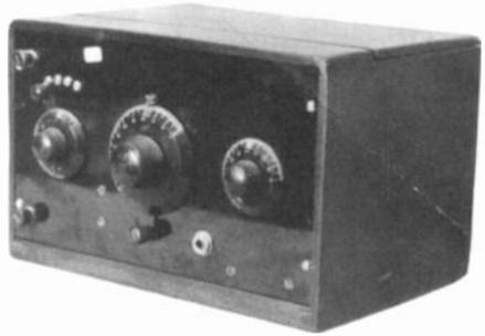
**TRI-CITY MANUFACTURING COMPANY MODEL W-4** – This 1923, roughly built 1-tube regenerative set has unique features on the panel. The tap switch shaft is concentric, with the knob controlling the spiderweb regeneration control. Connected below the tuning knob is a vertical bar attached to a much smaller knob. When this small knob is pushed down and turned to the left or right, it acts as a fine tuning vernier control. *(Walter V. Worth – Wollaston, MA)*
