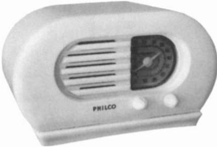
**PHILCO MODEL 42-KR3** – The chassis of this set is AC/DC and uses loktal type tubes, which are typical of Philcos of this era. At first glance, it would be easy to mistake this for a Bakelite set, but the cabinet is actually made of wood and painted ivory. Notice that the bottom of the base is curved slightly so that it could set on top of a refrigerator without rocking. Tops of refrigerators of 1942 vintage were slightly rounded. (Bill Harris – Roanoke, TX)
