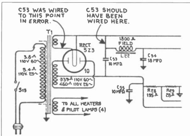
Figure 3. Partial schematic showing correct wiring of input filter capacitor.
