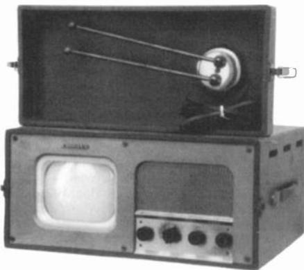
**CROSLY MODEL 9-425** – This 1949 portable television has a leatherette case, two chassis and 20 tubes. The antenna is attached to the front cover lid. (Tony and Lynn DeMara – Mt. Clemens, MI)
