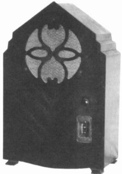
**U.S. RADIO & TELEVISION CORP. "SCREEN GRID" MODEL 27** – Schematically similar to the more popular Gloritone model, this 5-tube 1930 model has an inverted chassis. Oil-filled filter capacitors are enclosed in copper cans. *(Bob Lackey – Carlsbad, CA)*
