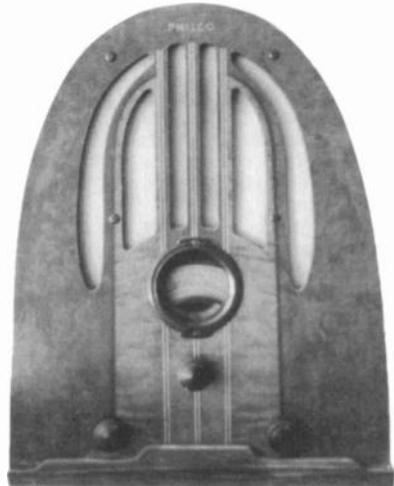
**PHILCO MODEL 37-34** – A 5-tube farm set with a vibrator power supply designed to be powered from a 6-volt storage battery, this 1937 cathedral works well. (Bill Harris – Roanoke, TX)
