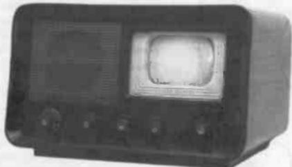
**PHILCO MODEL 48-700** – This 1948 7-inch set has only eight channels, but with changeable channel strips so that any channel from 2-13 could be added, depending on what area you lived in. This big and heavy set has 24 tubes and a 7JP4 picture tube. (*Tony and Lynn DeMara, Mt. Clemens, MI*)
