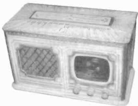
**EMERSON MODEL AM-187** – This AM/SW 5-tube set is in an antique white Repwood cabinet. The tubes used are Types 6A7, 6D6, 6Q7, 25L6, 25Z5 and a L49BG ballast. (*Joseph Kwoka – Delran, NJ*)
