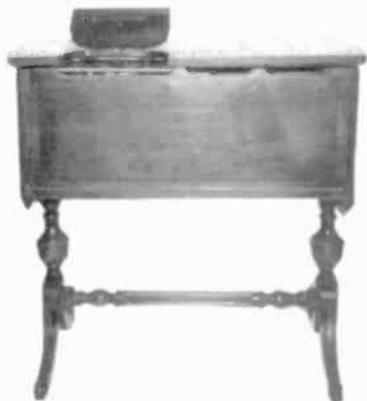
**MAJESTIC MODEL 15B** – This 5-tube superhet (which is called Fyfewood Model 154 in Rider's) uses tube Types 24 (2), 51, 47 and 80. In the front view, the lid over the controls is shown open. Note the stylish speaker grille in the end view. (*George Hausske – Wheaton, IL*)
