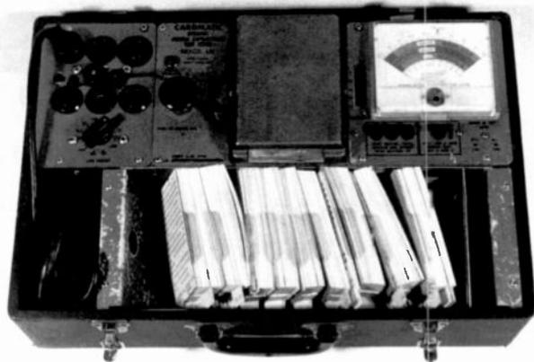
Figure 2. Hickok Model 121 Cardmatic dynamic mutual conductance tube tester.
