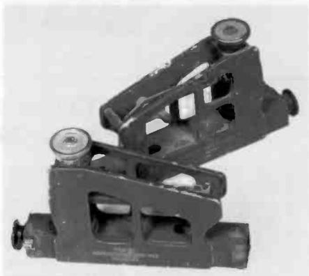
Figure 1. Atwater Kent Clinometers.
