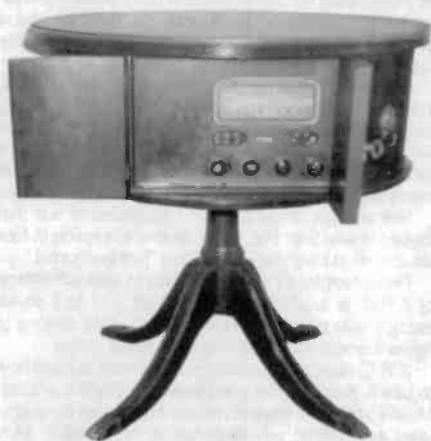
**BRUNSWICK MODEL 689** - This model is a 6-tube, 2-band, AC/DC set, made by RCA, housed in a Duncan Phyfe drum table. The cabinet has a lovely mahogany finish and features claw feet and "lion's head" drawer pulls. The sides are open shelves, and the front has two curved doors that open to reveal the radio controls. The self-contained loop antenna is wound onto the bottom surface of the drum. (*Irene M. and R. Edward Ripley - St. Paul, MN*)
