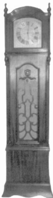
**STORY & CLARK MODEL C-108** – The cabinet of this sturdy grandfather clock radio is made of solid  $\frac{3}{4}$ " mahogany. The chassis is in two units, one mounted above the other. The schematic for this set appears in the "Miscellaneous" section of Rider's, Volume V, page 19. (*George Hausske – Wheaton, IL*)
