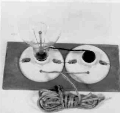
*Figure 1. Series light tester, a simple homemade device that will protect your radios and your house!*
