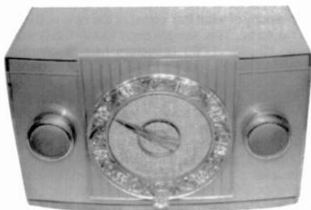
**CROSLLEY MODEL 11-113U** – The cabinet of this radio is made of clear molded plastic and is painted gold on the reverse side. The dial markings are silver colored. The radio is marked, "Made exclusively for the leading jewelers of America by Crosley." (*Cort and Eileen Ancman – San Antonio, TX*)
