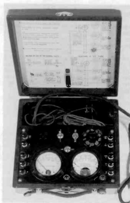
Figure 7. Weston Model 537 AC and DC radio set tester, a handy all-in-one set tester for early sets.
