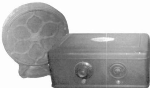
**ATWATER KENT MODEL 37** – This 1927 metal cabinet AC radio is shown with a working Atwater Kent Model E-3 cone speaker. (*Karen R. May – Los Angeles, CA*)
