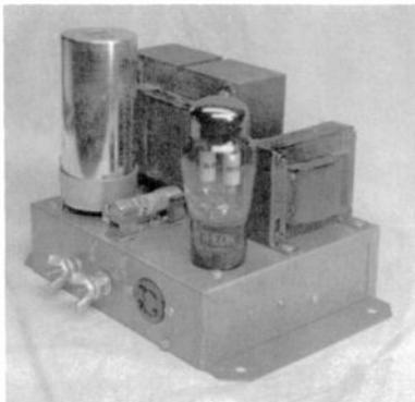
Figure 1. These power supplies operated from 6 volts DC for the mobile transceiver and probably supplied B+. Note the unusual rectifier tube used in both supplies.
