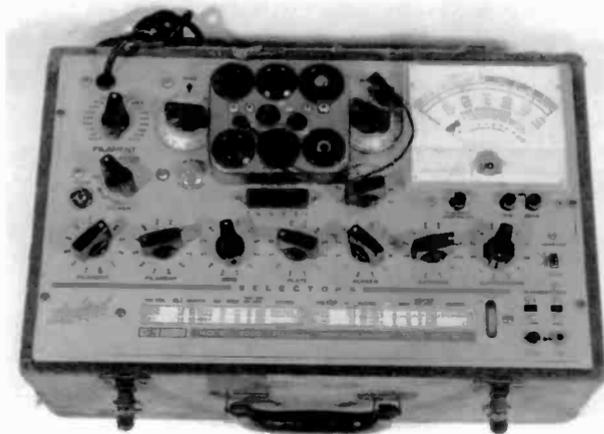
Figure 3. Hickok Model 6000 dynamic mutual conductance tube tester, one of the best for the vintage radio hobbyist.
