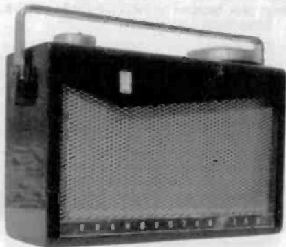
**SONY MODEL TR-72** - This 1958 transistor radio may be one of the first generation Japanese transistorized sets. It was made by Tokyo Tushin-Kogyo, which is presently Sony. This set uses 7 transistors, is powered by 3 "D" cells and is equipped with an oval speaker, ferrite bar antenna, and an earphone jack on the back. The cabinet is wooden, with a piano-hinged back and leather pull tug. (*Hideo Sasau - Tokyo, Japan*)
