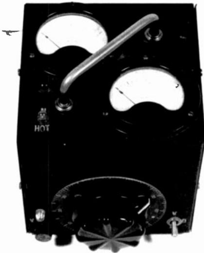
Figure 5. A Variac. Note the volt and ammeters and the fuse protection. There are 2 plugs mounted on the back.
