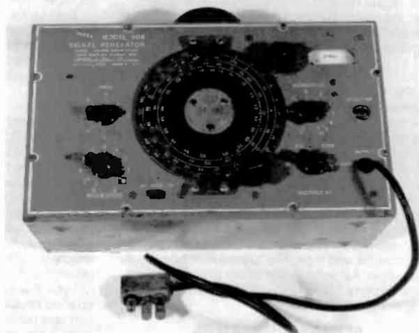
Figure 4. McMurdo Silver Model 906 signal generator.
