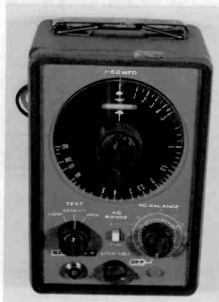
Figure 6. Eico Model 955 in-circuit capacitor tester.
