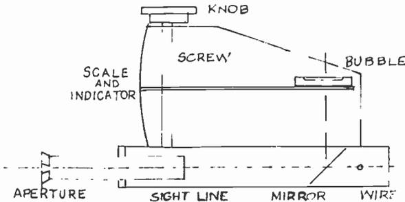
Figure 2. A simplified diagram of the Atwater Kent Clinometer.
