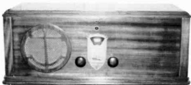
**UNITED AMERICAN BOSCH MODEL 84** – This "motor boat" radio was designed especially for use on motor, auxiliary or sail yachts. It was made in 1933. (*Bob Molesworth – New Britain, PA*)
