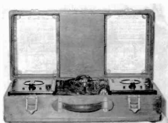
Model 664 – An AC volt capacity meter, standardized date 1930, and Model 665 – A DC VOM, standardized date 1935. Although sold separately, these models were packaged together in a Type CV case as a test repair kit.
