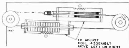
Figure 3. Tuning mechanism used in Airline Models 04BR-515A and 04BR-515B and in Belmont Model 533. (Rider's)
