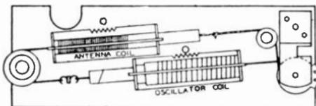
Figure 8. The tuning mechanism used in the Belmont Model 4BA1. (Rider's)
