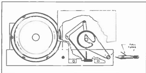
Figure 9. The tuning mechanism used in the Detrola Model 571X. (Rider's)
