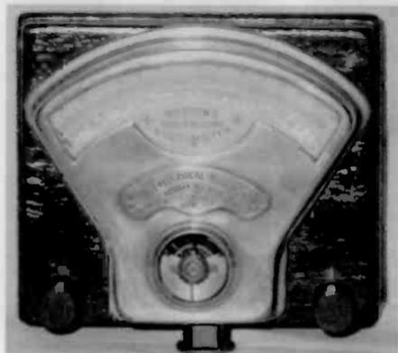
Model 1 - A voltmeter, one of the first Weston meters built, patent date 1888.
