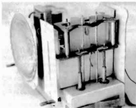
Figure 5. View of chassis and tuning mechanism in Airline Model 84KR-1520A.
