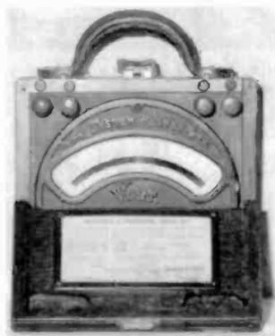
Model 45 – An early System Weston DC voltmeter, last patent date 1898.
