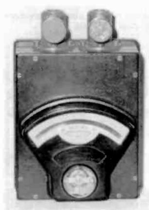
Model 1 – A direct reading ammeter, last patent date 1906.
