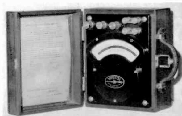
Model 370 – An AC/DC ammeter, standardized date 1916. The instruction sheet is attached to the inside of the cover lid.
