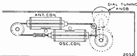
Figure 7. Typical Belmont permeability tuning mechanism. (Rider's)
