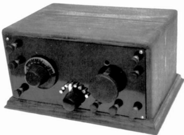
Figure 1. The restored Eaton single circuit set.
