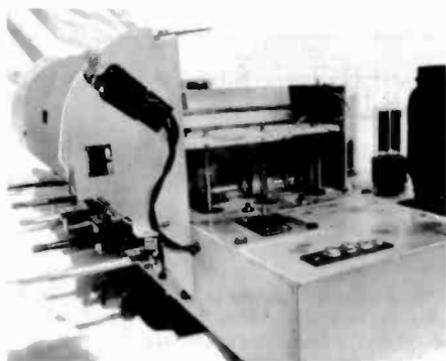
Figure 2. Admiral Model 6C71-10A1 chassis with a view of the tuning mechanism.
