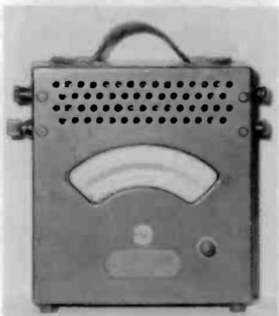
Model 155 - An AC voltmeter, last patent date 1898.
