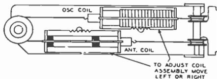
Figure 6. The tuning mechanism used in the Belmont Models 151 and 536. (Rider's)
