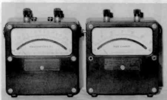
On left: Model 430 - A DC milliammeter of WWII vintage. On right: Model 756 - A foot candle meter, date unknown.
