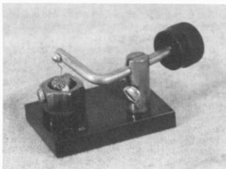
Figure 6. The Electro-Importing Co. type crystal detector.
