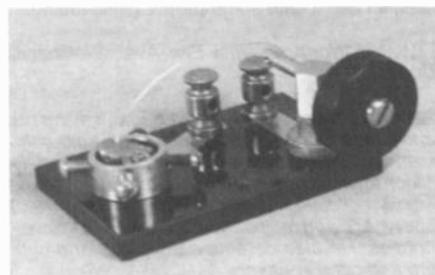
Figure 3. The Grebe type crystal detector.
