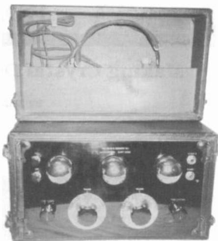
**KENNEDY MODEL III PORTABLE** – This 1924 set is similar to the Kennedy Model V. The case is covered with a black, grained fabric. Note that the earphones fit inside the lid. (*Ed Bell – Raleigh, NC*)
