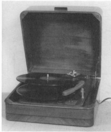
Figure 5. Motorola wireless record player with a record changer.
