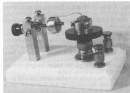
Figure 5. The Duck Type G crystal detector.
