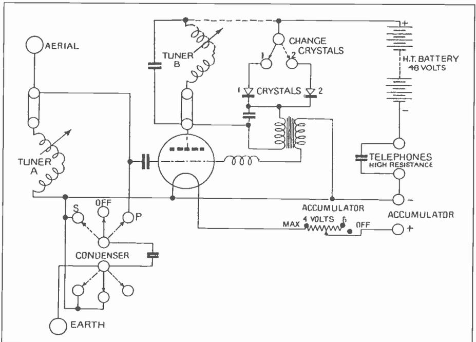
Figure 4. Circuit Diagram of the B.T.H. Valve-Crystal Receiver, Type VC. (Source: H.M. Dowsett, "Wireless Telephony and Broadcasting Volume II," copy courtesy of C.F. Crandell.)
