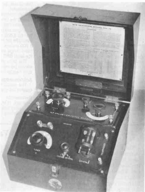
Figure 1. The B.T.H. Radiola I Type VC, Form 'B' Receiver.
