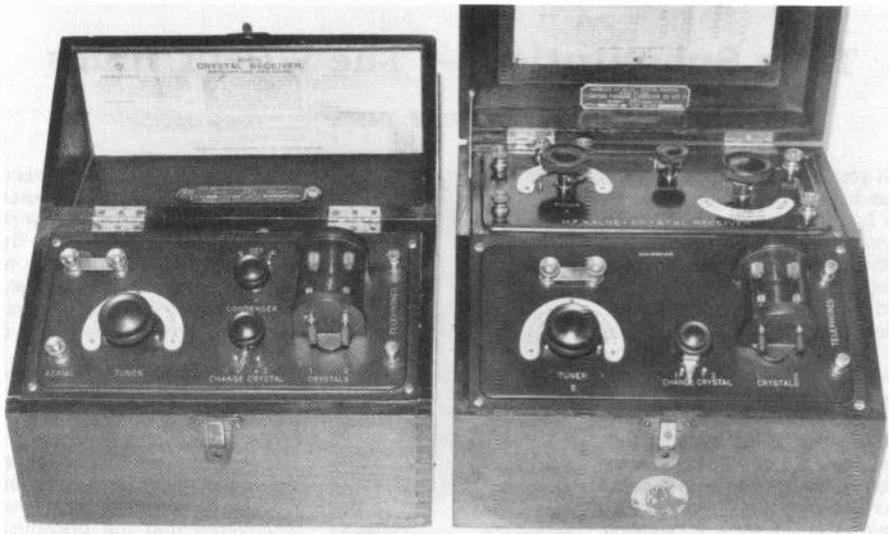
Figure 3. The Type VC, Form 'B' Receiver, right, and the earlier Padiola Type C Crystal Set, left. Note the similarity of the front panels.
