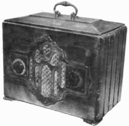
**AIRLINE MODEL UNKNOWN** – This 5-tube mantel radio appears to be circa 1933. Its tube complement is (1) 6C6, (2) 6D6, (1) 43, and (1) 25Z5. It has a heater strip resistor mounted to the back of the chassis instead of a line cord resistor. (*Robert and Shirley Schafbuch – Carrollton, KY*)
