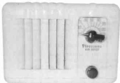
**FIRESTONE AIR CHIEF MODEL S7425-4** – The dimensions of this tiny, white plastic set are 6½" wide x 4½" high x 4½" deep. Manufactured ca. 1938, the set uses Types 6K7, 6J7, 25L6, and 25Z6 tubes, plus a resistance line cord. (Stanley Lopes – Concord, CA)
