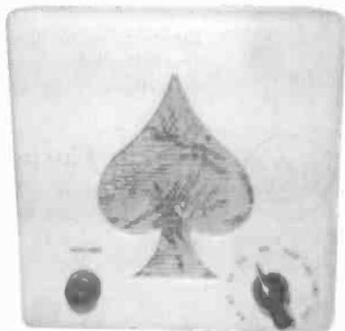
**SETCO MODEL NUMBER UNKNOWN** – This "ace" of a radio was made in Minneapolis, Minnesota, circa 1939. The cube-shaped cabinet, 6" x 6" x 6", contains an AC/DC chassis with 5 loktal tubes and inductance tuning. (Jimmy Downes – Covington, LA)
