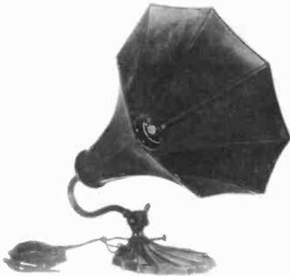
**TELEMACO TELEPHONE MAINTENANCE CO. MODEL TH-1** – Utilizing a type of folded horn design, the driver faces the inside of this horn. The driver adjustment knob is easily accessible, and the cast-iron base includes a provision for raising and lowering the listening angle. For the space-conscious buyer, this little horn measures 11½" long x 10½" diameter. (*Robert Bailey – Jacksonville, FL*)
