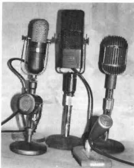
Figure 2. An assortment of familiar studio microphones. Clockwise from lower left: a Turner U9S, an RCA 77DX, an RCA 44BX, an Altec 639A, and an RCA BK-1A.
