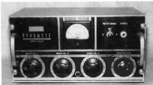
Figure 4. A relatively compact tube-type Gates "Dynamote" remote amplifier mixer.
