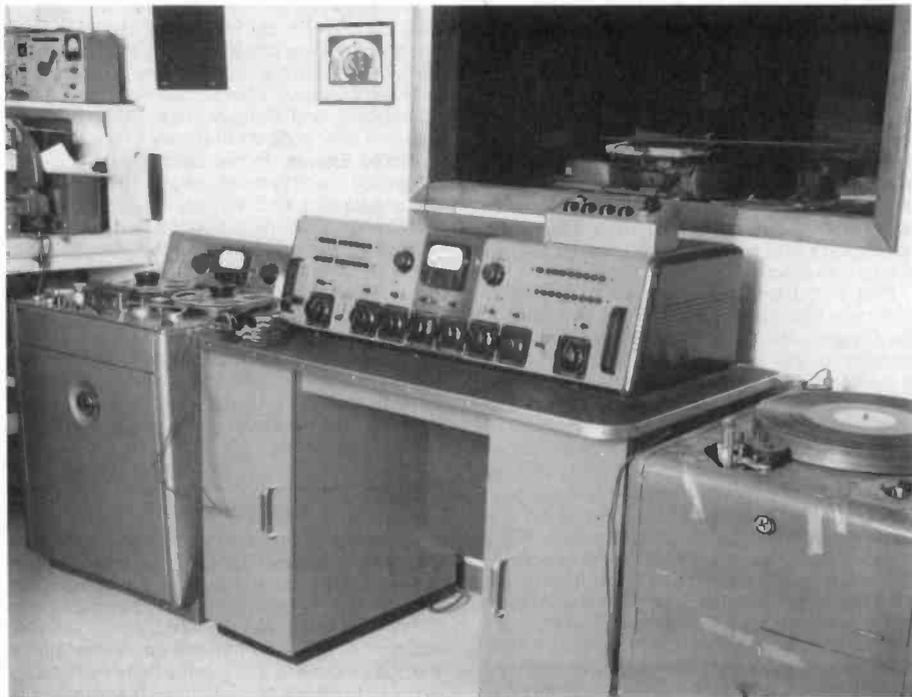
Figure 1. An RCA 76-B2 console (center), with an Ampex 300 tape deck (left), and a 16-inch transcription turntable (right).
