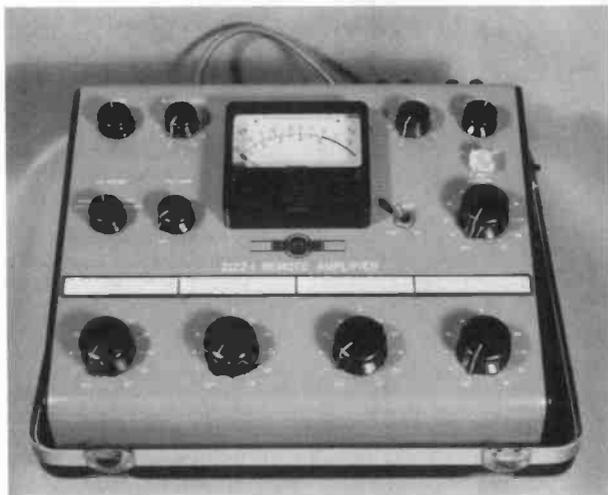
Figure 5. A Collins lightweight solid-state remote amplifier.
