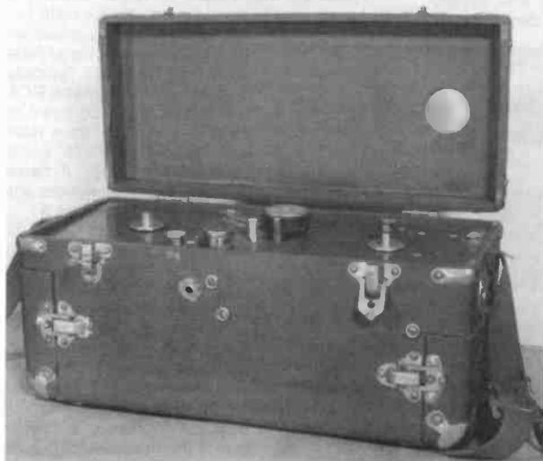
Figure 3. A Stancil-Hoffman portable reel-to-reel tape recorder.
