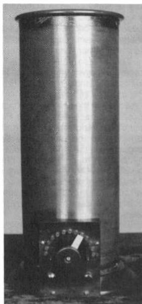
Figure 8. The loading inductance coil used in the Type 93 long wave receiver.
