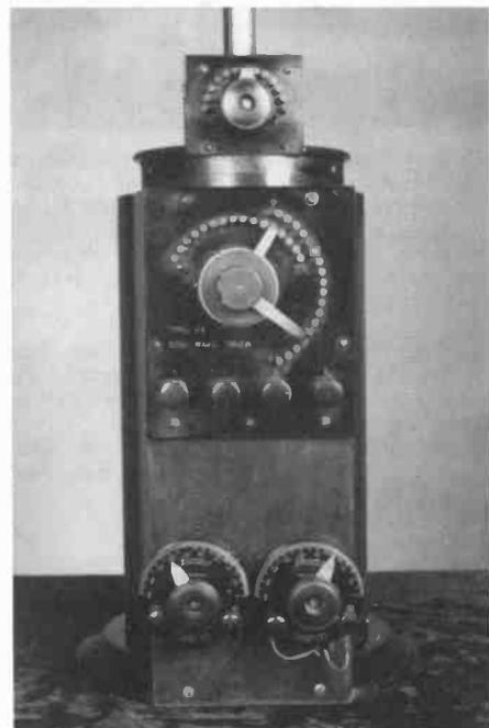
Figure 3 Panel view of the Type 94 long wave receiving transformer.
