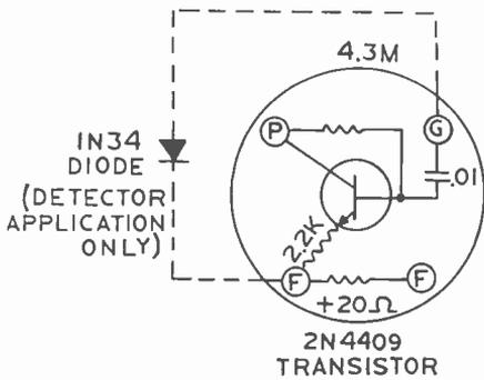
Figure 2. Diagram for a solid-state substitute for a Type 201-A tube, according to Jacob Anthes.
