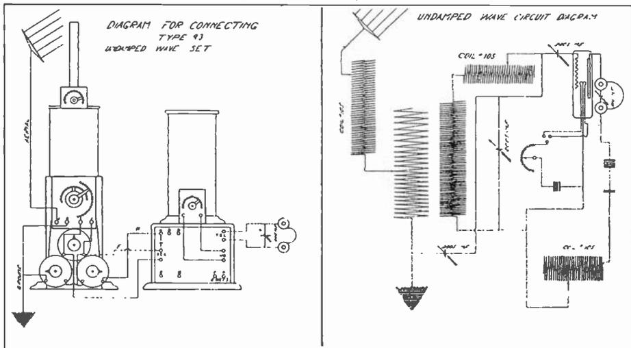
Figure 9. Schematic diagram for the Type 93 long wave receiver from a Radio Apparatus Company catalog.
