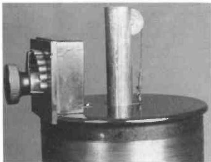
Figure 4. Close-up view of the pulley mechanism for the Type 94 receiving transformer counterweight.
