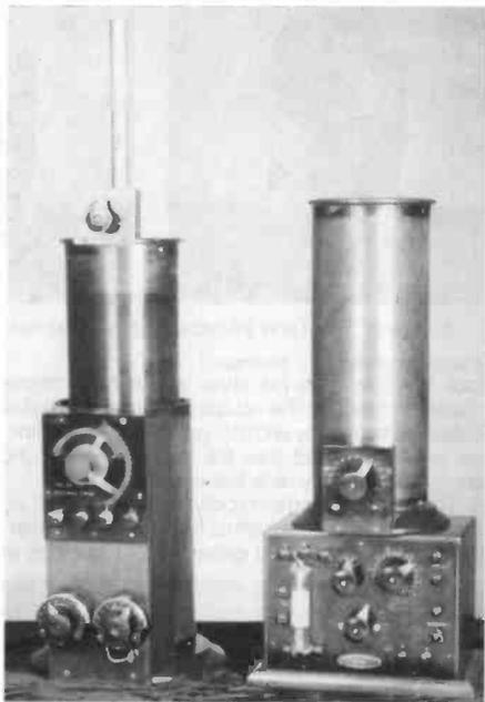
*Figure 1. The Type 93 long wave receiver in Ron Frisbie's collection. When purchased, the receiving transformer on the left did not include the two variable capacitors seen on the lower portion of the panel. Ron has added RCA Faradon capacitors until he can replace them with original Radio Apparatus Company capacitors.*
