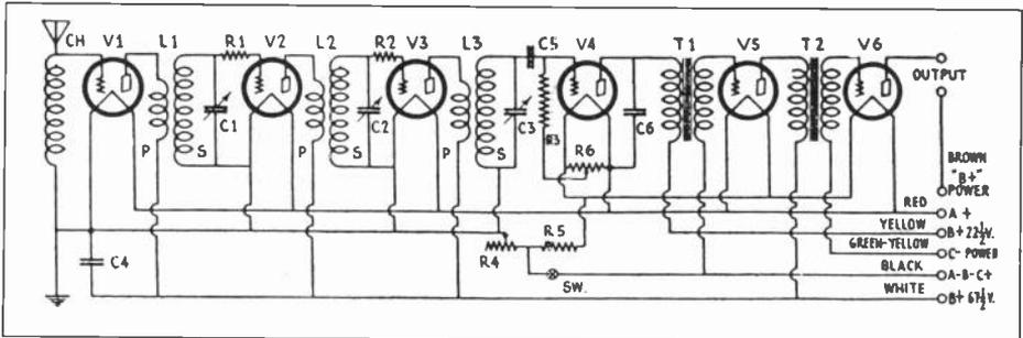
Figure 4. A schematic for a typical 1920s radio circuit.
