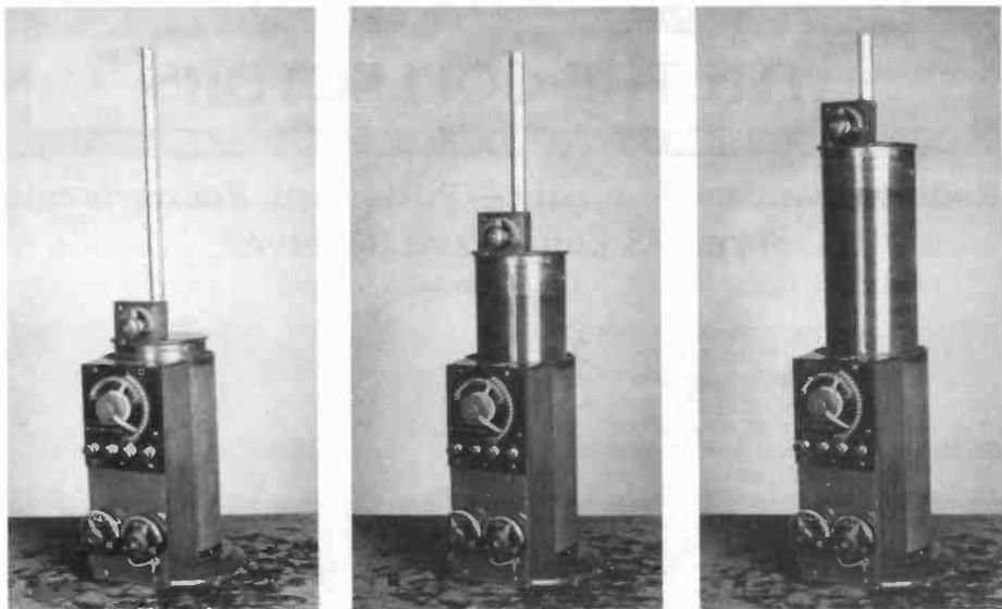
Figure 2. The Type 94 receiving transformer in closed, half-closed, and fully extended positions.
