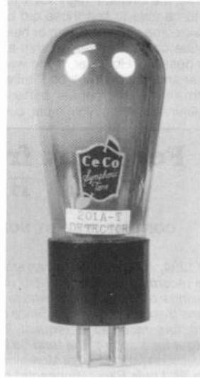
Figure 3. A converted solid-state CeCo Type 201-A tube which can be used as a detector.
