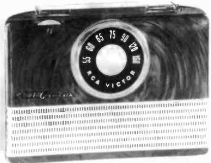
**RCA VICTOR MODEL B-411** – This stylish 1940s portable radio is made of marbled brown plastic and brushed aluminum. It has a standard broadcast, 4-tube chassis which used one 1½-volt battery and one 67½-volt battery. Currently, it is comfortably stuffed with 9-volt batteries and a flashlight battery, giving it a new lease on portability! (*Robert Bailey – Jacksonville, FL*)
