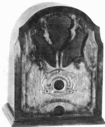
**JEFFERSON CATHEDRAL MODEL UNKNOWN** – This is a low-priced junior cathedral radio from the 1930s. The brand name "Jefferson" is on the dial escutcheon; however, there is no manufacturer ID or model number on its 4-tube chassis. The cabinet is made of inexpensive wood, enhanced with groove carvings and toning lacquer. This set measures only 12¾" tall and 9½" wide. (Robert Bailey – Jacksonville, FL)
