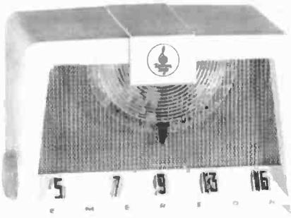
**EMERSON MODEL 810** – This 1955 Emerson has a typical 5-tube AC-DC chassis. The dial pointer at the top of the radio is mounted behind a plastic apron and aims downward at the numbers below. (*Robert Bailey – Jacksonville, FL*)
