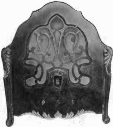
**OZARKA VIKING 92** – This Gothic-styled cathedral was made by Ozarka in 1931. The escutcheon has the name "Viking" on it in a cloisonne finish. The chassis contains a 7-tube TRF circuit. (*Greg Farmer – Gridley, MN*)
