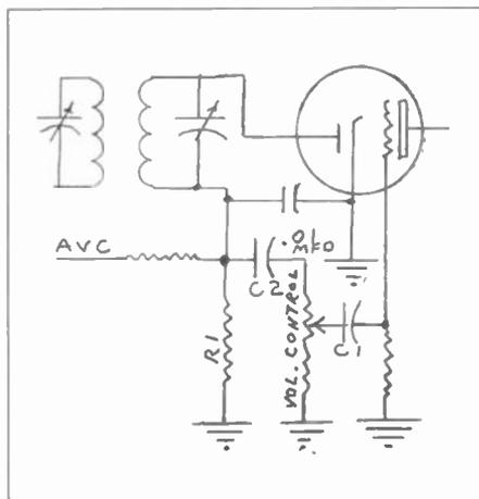
Figure 2. A circuit modification to cure a noisy volume control.
