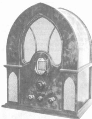
**PHILCO MODEL 610 IN HOME-BREW CABINET** – The electronics of this set is an original Model 610 5-tube superheterodyne with BC and SW, 115-VAC. The after-market cabinet, designed and manufactured by "G.V.R." in Marina, California, is made of walnut with a walnut burl front and lacewood veneers over plywood. This set should alert collectors to newer home-brew creations coming into the market. (Glen Johnson – Marina, CA)
