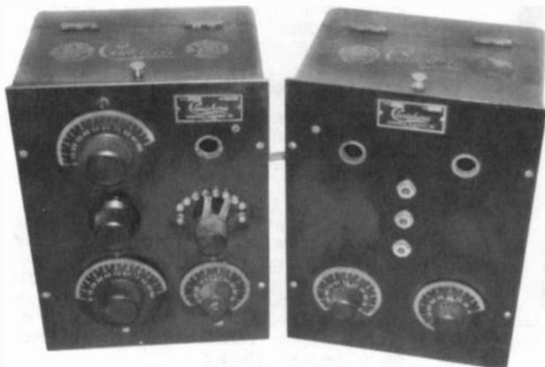
**CLARIPHONE MODEL UNKNOWN** – These detector (left) and amplifier (right) units were made by Campbell Electric Co. in Lynn, Mass., probably in 1922. According to the Lynn Historical Society, Campbell made electric and magnetic apparatus. Campbell's radios appear to be very rare. Any others? (Merrill Bancroft – Townsend, MA)
