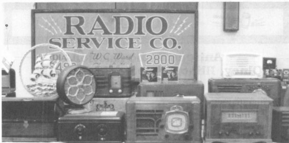
Figure 2. An assortment of radios and speakers, including a 1927 Tower Adventurer cone speaker and an Atwater Kent Type E speaker on an AK Model 37 radio.
