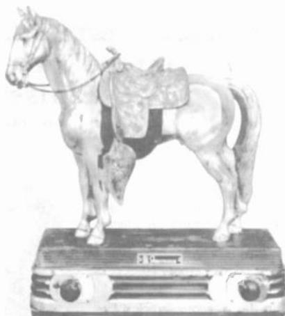
**ABBOTWARES MODEL Z477** – This copper-plated, diecast metal radio has a standard 5-tube AC/DC chassis. The speaker is mounted face up in the top of the base. The saddle and blanket are removable. (Herbert H. Eitz – Juniata, NE)
