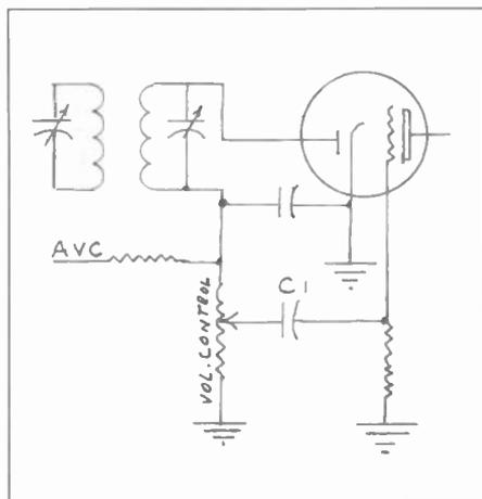
Figure 1. A common volume control circuit.
