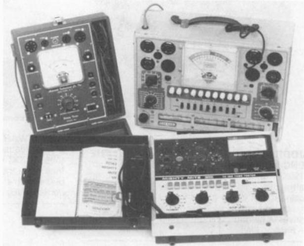
*Figure 1. Hickok testers were very expensive and many servicemen made do with emission testers like these: the Sencore Mighty Mite VII TC162 (bottom), and the Jackson dynamic tube tester (upper right). The Accurate Model 161 (upper left) is merely a heater filament continuity checker.*
