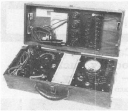
Figure 4. This Triplet test oscillator and set analyzer, mounted in a portable case, has test sockets for 4-, 5-, 6-, and 7-pin tubes and contains a multimeter.
