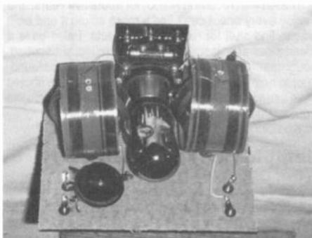
Figure 2. An internal view of the Echophone Model 7 repro.
