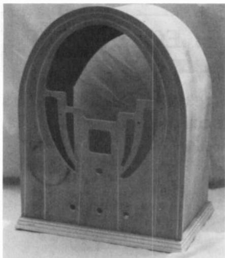
Figure 4. The cabinet completed with base trim cut on an angle from  $\frac{3}{4}$ -inch spruce.
