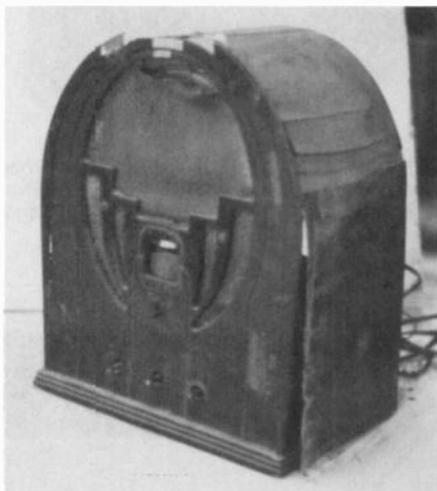
*Figure 1. The sadly deteriorated Philco 60 as found, but with knobs and dial escutcheon removed.*
