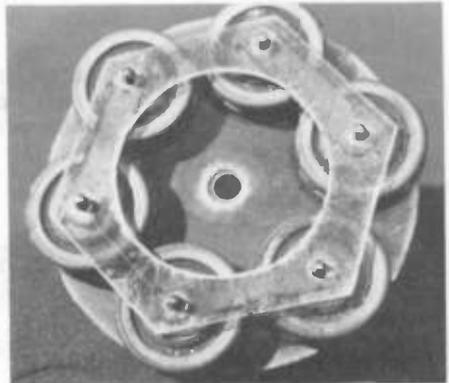
Figure 7. Removal of the diaphragm reveals another mica spacer and 6 carbon buttons. These buttons are probably of the Monarch brand.
