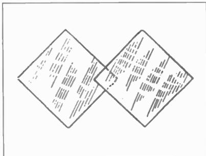
Figure 3. This unusual set of condenser plates will produce straight-line wavelength tuning.
