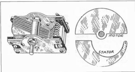
Figure 5. A version of a straight-line frequency tuning condenser that is much smaller than the unit shown in Figure 4. Note the semi-circular rotor and the odd shaped stator.
