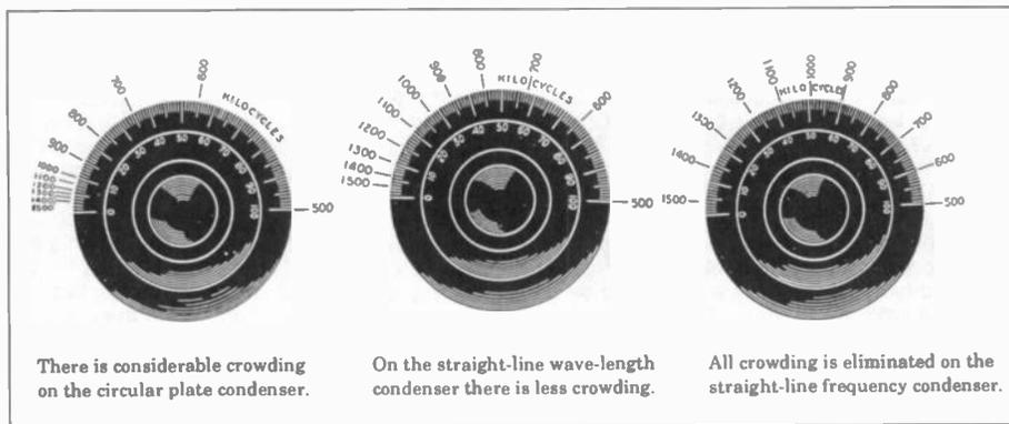
Figure 1. Examples of the relationship between tuning capacitor type and dial calibration.
