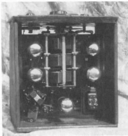
Figure 3. Top view of the Magnavox showing the tubes, 3-gang condenser, and audio transformers.
