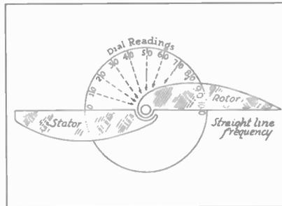
Figure 4. A straight-line frequency tuning condenser with plates that are much longer than the other two types of tuning condensers.
