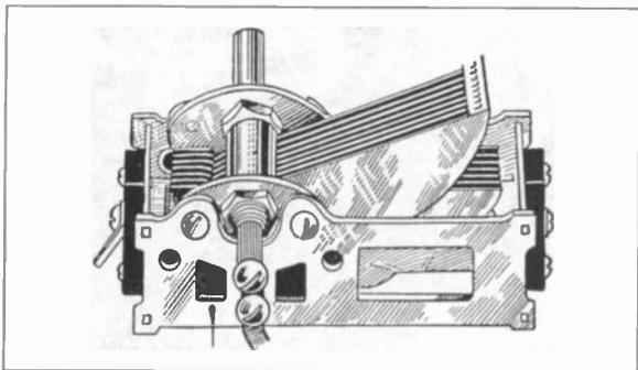
Figure 8. A modified straight-line frequency condenser that combines SLF and SLW characteristics.
