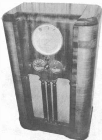
**NORTHERN ELECTRIC MODEL 1121A** – This 11-tube Canadian radio tunes the BC band, the police band, and 3 SW bands. It features bandspread tuning on the SW bands and AFC on the BC band. A "fidelity control switch" controls the selectivity of the two IF stages. (*Marcel La Bossiere – Marmora, Ontario, Canada*)
