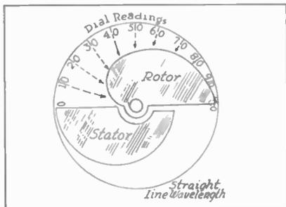
Figure 2. A straight-line wavelength tuning condenser with its shaped plates. Note the position of the rotor plates in relation to the dial reading.
