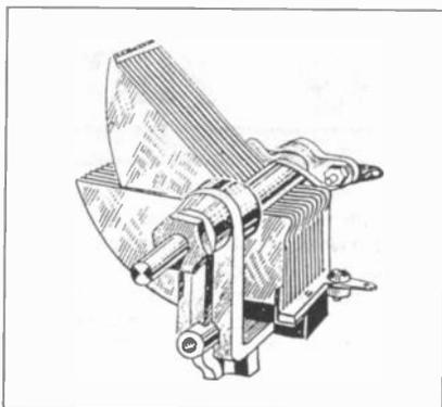
Figure 6. Another version of a straight-line frequency tuning condenser that results in a smaller width by the use of a greater number of smaller plates.
