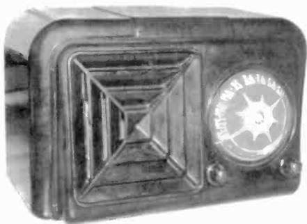
**AUTOMATIC MODEL 614X** – This 1946 AC/DC superhet was manufactured by the Automatic Radio Co., Boston, Mass., and uses the following tubes: Types 12SA7GT, 12SK7GT (2), 12SQ7GT, 35L6GT, and 35Z5GT. The cabinet is brown Bakelite and features a rather unusual "starburst" dial. (Douglas Fox – St. Charles, IL)
