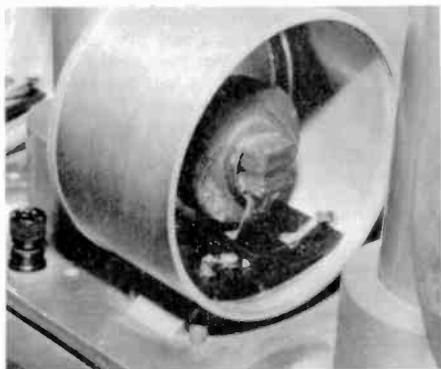
Figure 6. One of the iron-core IF transformers and its machined aluminum cans with the cover removed.
