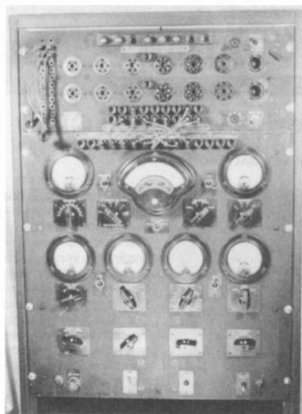
Figure 1. This Weston laboratory tube tester sports enough testing capability to satisfy even the owners of tube-operated, high-fidelity audio amplifiers.
