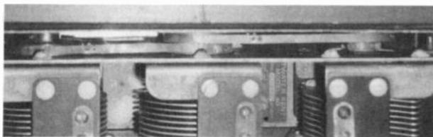
Figure 8. The upper portion of the photo shows both copper belts in place. These belts are properly seated over the pins on the pulleys of the three variable condensers in the lower portion of the photo. Note the old solder splice, still intact, on the bottom belt, in the center of the photo.
