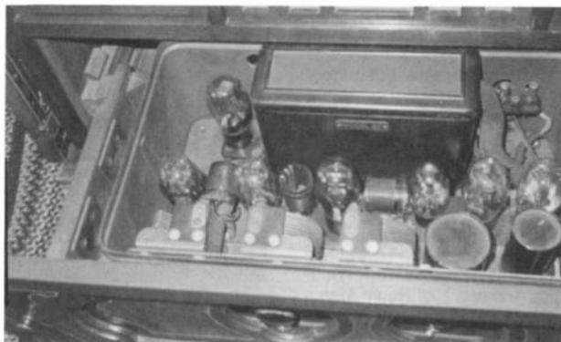
Figure 5. The sliding drawer gives easy access for tube testing and for measuring power supply voltages. The power supply terminals are accessible when the power supply lid is removed.
