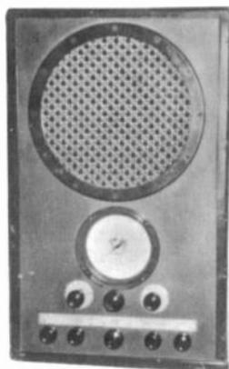
**RCA MODEL AVR-5** – This 1934 communications receiver has 9 tubes, AF and RF gain controls, a CW oscillator, and a 10" speaker. It receives 150 Kc to 18 Mc. The unusual wooden tombstone-style cabinet stands 22" high. (*Frank Franowsky – Santa Fe, NM*)
