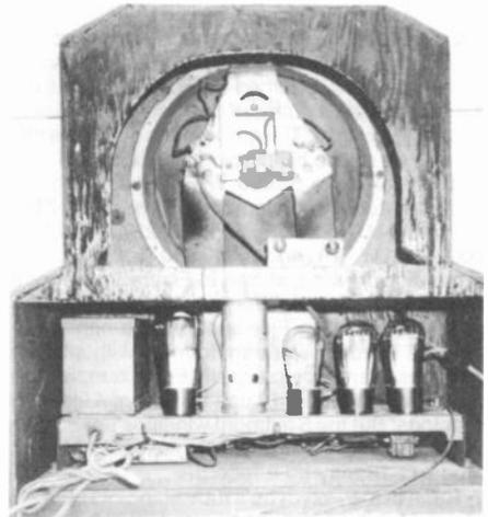
Figure 4. A rear view of the Polydyne shows the 10" magnetic speaker and the chassis.
