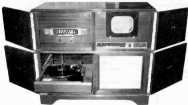
MAJESTIC MODEL 18C91 — This is a 1948-1949 console combo with a 7" TV screen. It has two separate chassis, one for the AM/FM radio/phono and one for the TV. This set uses a Type 5U4 rectifier and power transformer for the low voltage power supply. The high voltage is RF type with a small 6C4 overworked as a self excited oscillator output for high voltage. The automatic turntable is 78 rpm only. Everything is in working condition. (Hicksville Radio & TV — Hicksville, NY)
