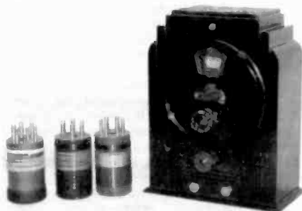
ICA UNIVERSAL "MASCOT" — This very small, 1-tube radio uses four plug-in coils to cover BC and SW bands. The batteries are externally connected by a cable. The headphones plug into the two jacks at the base of the Bakelite case. (Wally Worth — Wollaston, MA)
