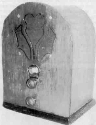
**MERCURY RADIO CO., N. Y., MODEL UNKNOWN** - This 4-tube cathedral, ca. 1932, has a plywood case. The chassis and speaker are very heavy. I also have a very heavy Mercury cygnet horn speaker named "Grand" from the same company. (*Wally Worth - Wollaston, MA*)
