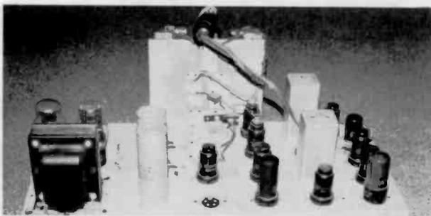
Figure 1. The 15-tube chassis of an Emerson Model X183.
