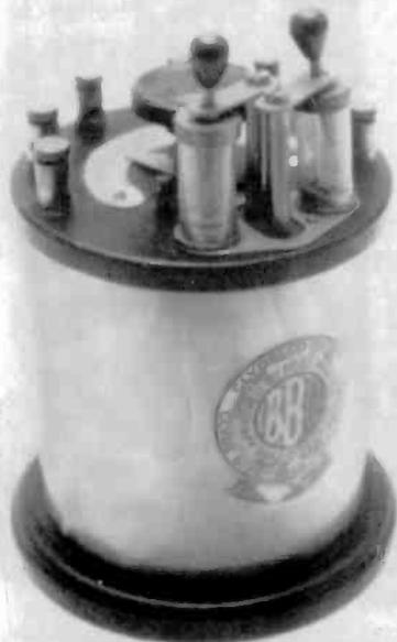
**CLYDELCO CRYSTAL SET** – This double glass-enclosed catwhisker and galena crystal set was manufactured by the Clyde Electrical Co. in 1923. The tuning variometer, enclosed in celluloid below the top panel, has the GPO (Government Post Office Approval) No. 871. It is one of my most interesting crystal sets from Great Britain. (Erwin Macho – Vienna, Austria)
