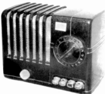
**SILVERTONE 6102A** – This 5-tube, black Bakelite set, ca. 1959, has the grille running up the front, over the top, and down the back, similar to the Airline Model 83-BR-351A by the Belmont Co. The case lifts straight off the chassis. (*Wally Worth – Wollaston, MA*)
