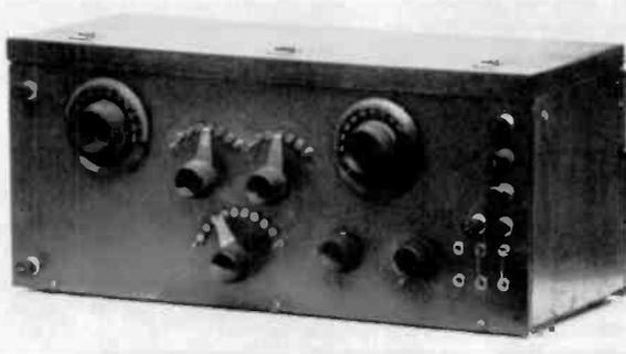
Figure 3. The 2-tube Reinartz receiver.
