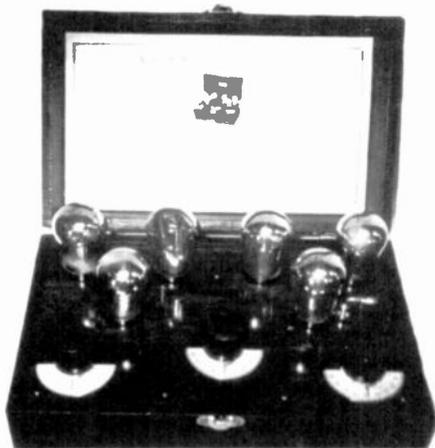
**A-C-S RADIO RECEIVER** – This compact 6-tube radio was manufactured by the Multiple Selling Corp., Madison Ave., New York City. It features "No Solder" electrical connections using copper strips. Its size, with cover closed, is 7" x 13" x 7 1/4". It has many similarities, especially the dials, to that of the Martian "Beauty" 1-tube set. If anyone has any information about this receiver or the manufacturer, please write A.R.C. (Ed Bell – Raleigh, NC)
