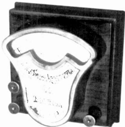
**KNOTT STUDENT'S AMMETER** – This beautiful example of laboratory equipment was manufactured by the L.F. Knott Apparatus Co. of Boston. The thick mahogany board, heavy metal casting, and rugged binding posts helped it survive rough handling in the laboratory since the early 1900s. (Dave Crocker – Mashpee, MA)
