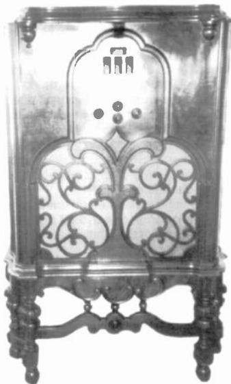
**ZENITH MODEL 618** – This Gothic 8-tube superhet has a look unlike many 1930s Zeniths I have seen. It has two speakers and three bezel openings for tuning. (Joe Beckley – South Port, NC)
