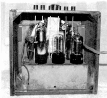
Figure 2. Rear chassis view of the RCA 94X2, showing the push buttons projecting through the top of the cabinet.
