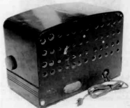
Figure 2. Rear view of the RCA 5Q8 showing the original fiberboard back cover.
