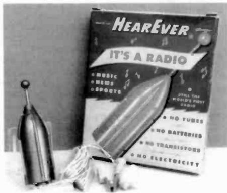
**HEAREVER MODEL 20** – This rocket-shaped, germanium crystal radio tunes by moving the nose rod on the front of the rocket. The claim on the front of the original box says: "Still The World's First Radio." (*Harry Blesy – Hindsdale, IL*)
