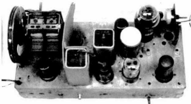
Figure 3. The chassis of the RCA 5Q8 removed for inspection.
