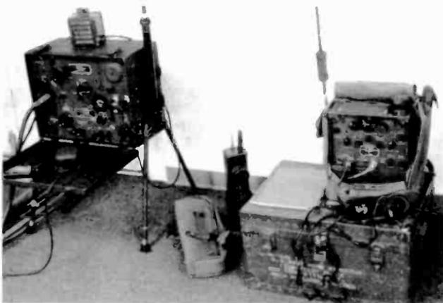
A U.S. Navy TBY set on display at right with a U.S. Army BC-611 HT at left. The CRI-43044 transceiver operates from about 28 Mc to 80 Mc for short distance work. Output on CW is about 3/4-watt and 1/2-watt on phone. At far left, is an Army SCR-284 field set.
