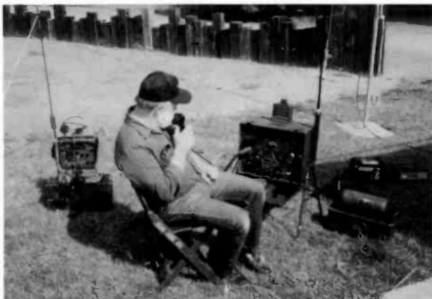
Tom Horsfall, WA6OPE, working the SCR-284 with a Navy TBY in back. Note the PE-103 dynamotor supply for the HF set.
