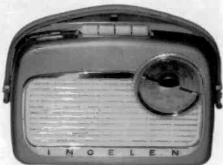
**INGELEN MODEL TRV-111** – This 1959 portable, made in Austria, was a very popular radio. It operates on battery power and tunes only the AM band. The case is green leatherette. (Erwin Macho — Vienna, Austria)
