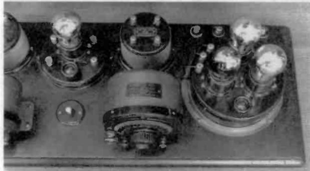
*Figure 6. A view showing the multiple use of binding posts on the components on the right side of the Radiodyne receiver.*
