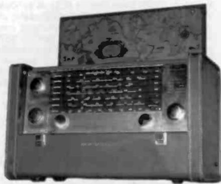
**RCA MODEL 3-BX-671 STRATO-WORLD** – This 1954 AM/FM portable radio is RCA's answer to the Zenith Trans-Oceanic. It is a 7-band receiver with separate bass and treble controls. The case is leather and has a world map in the lid. I found it with its original instruction book. (William Dalton, Jr. — Bridgeport, CT)
