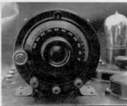
*Figure 8. One of the Radiodyne tuning condensers showing the binding posts at the bottom.*
