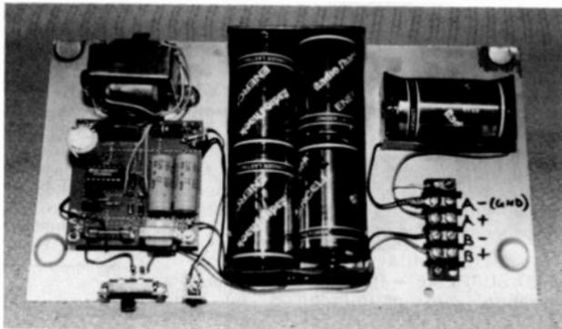
Figure 1. The completed A and B power supply, including the D cells.
