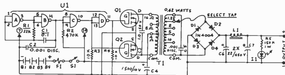
Figure 2. Schematic diagram for DC-to-DC B supply.
