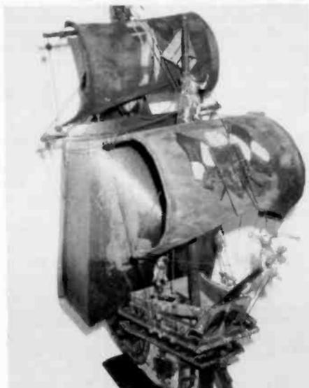
Figure 2. Another view of the "Venetian Lepanto" ship model cone speaker showing the cast metal figures, painted sails and bow (front) details.
