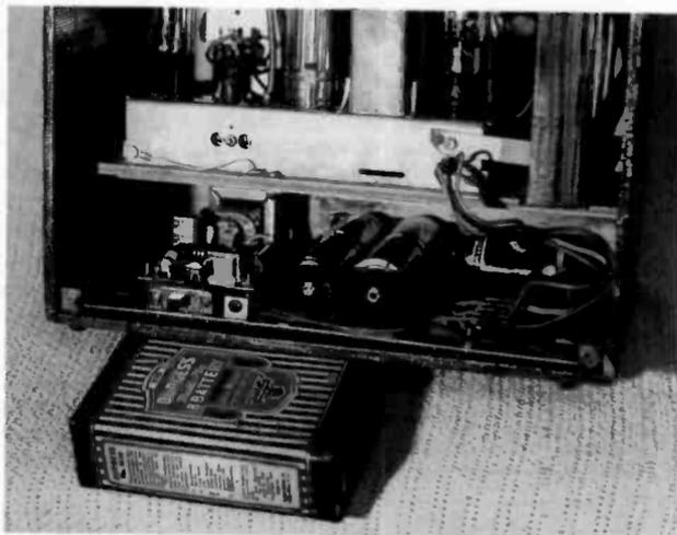
Figure 4. A prototype of the supply mounted in the battery compartment of the RCA Model BT-40 portable radio.
