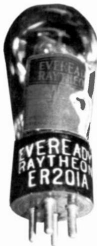
Figure 2. In addition to the marking on the tube's plate, and the printing on the paper label, the tube's base is branded "Eveready Raytheon ER201A."
