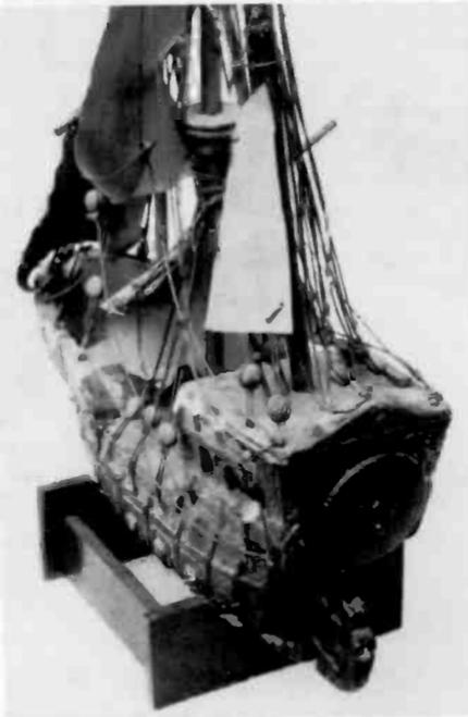
Figure 8. The rear view of the plaster ship model speaker, showing how the horn speaker driver fits into the rear of the hull. The driver is quite obviously a Utah unit.
