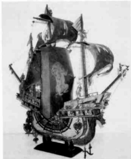
Figure 1. The very colorful cone speaker ship model "Venetian Lepanto" made by Miniature Ship Models, Inc., of Philadelphia. The sail with the lion design painted on it is the cone speaker. Look carefully and you will see the sailor figurines in the rigging.
