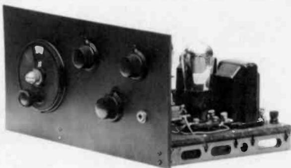
Figure 1. A front view of the restored shortwave Pilot Wasp.
