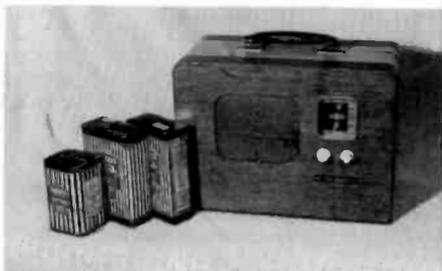
Figure 5. The BT-40 with the battery complement originally required for battery operation.
