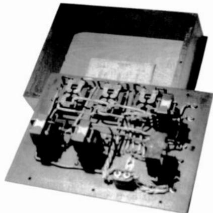
Figure 2. Internal view of the Western Electric 7A amplifier.
