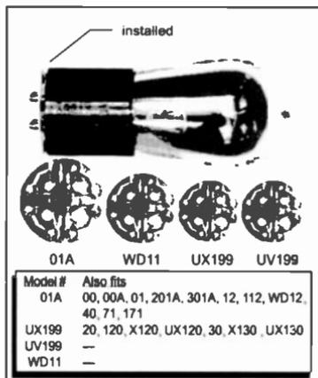
These tube repair wafers are solid-state devices for quick and easy repair of early vacuum tubes. The wafer is installed by simply sliding it over the tube pins and reinserting the tube into its socket. If the filament is intact, but there is little or no emission, the filament may be lit for best visual effect. However, the tube can be open filament.
