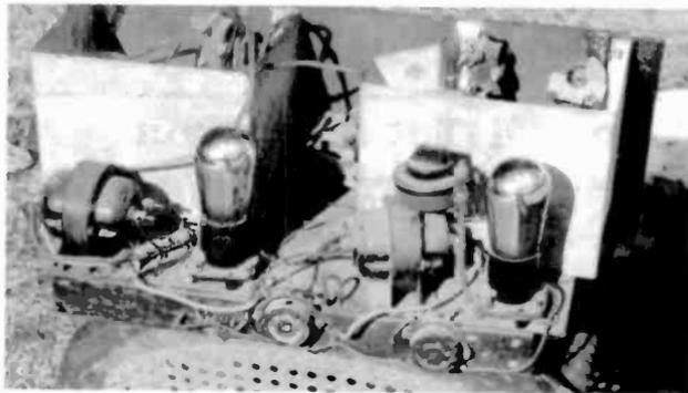
Figure 3. The home-brew version of the Super-Wasp in its "as found" state.
