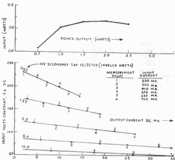
Figure 3. Efficiency curve for the DC-to-DC Converter.
