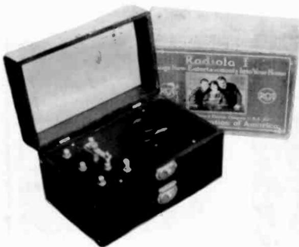
**RCA RADIOLA I** – This rare perikon crystal set was found in its original box! It also came with the original Murdock Type 56 headphones in the back compartment. With "Radiola I" on the panel, this is the later version of the two sets designated by RCA as the ER-753A. The earlier version has the RCA "World-Wide Radio" logo on the panel. Both versions were offsprings of the 1922 Model ER-753, which was sold in a metal wedge-shaped box. (Dave Crocker – Mashpee, MA)
