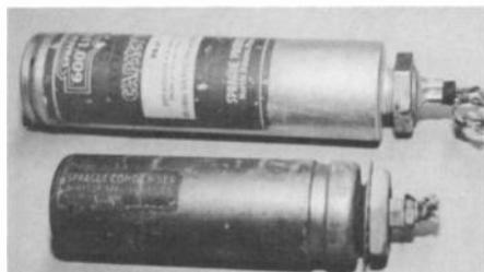
Figure 6. Two examples of can-type electrolytic capacitors: a wet type at the bottom and a dry type at the top. Note the nut and threaded base used to mount the capacitors.
