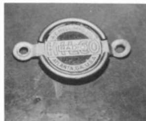
Figure 3. This "Hilco" mica capacitor has a very colorful label, and its round case is unusual.
