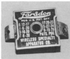
Figure 2. This "Faradon" mica capacitor carries patent dates ranging from 6-12-17 to 9-15-25.
