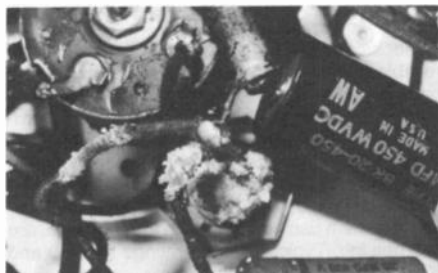
Figure 7. An example of a leaking wet electrolytic capacitor.
