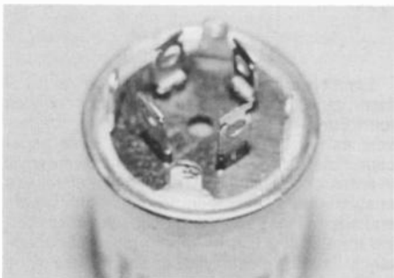
Figure 10. This "bottoms up" view shows a 4-section electrolytic capacitor.
