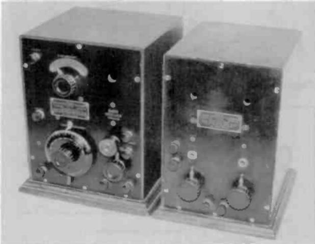
Figure 3. Front view of the SC-10 receiver and the Type S amplifier.
