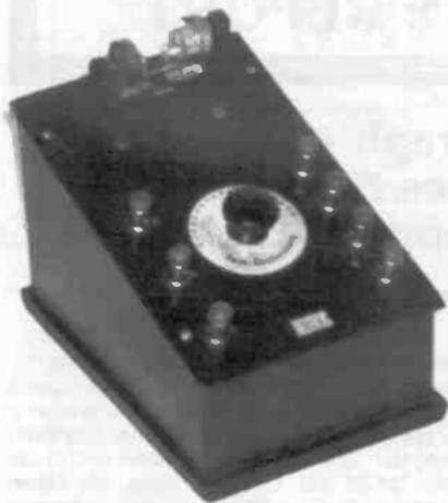
**EUMIG CRYSTAL SET** – This is one of the earliest sets from the Eumig factory in Vienna. It was built in 1924 and has slide tuning. The plug-in crystal detector is labeled “King.” (*Erwin Macho – Vienna, Austria*)
