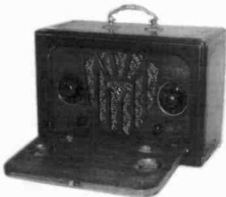
**SPARTON MODEL N-61** – This tiny, 1933, 5-tube radio, only 7" tall and 9 $\frac{3}{4}$ " wide, is housed in a cherry wood case with pull-down front. The decorative handle on top is made of brass. (*Wally Worth – Wollaston, MA*)
