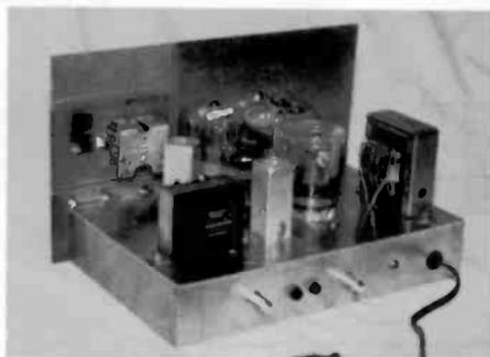
Figure 5. The Multivalve Receiver No. 2, using a Type 14BR11 Compactron in a straight TRF circuit.
