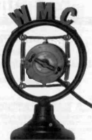
**WESTERN ELECTRIC MODEL 387W MICROPHONE** – This 1920s double-carbon, spring-type microphone was used in the early days of broadcasting. Radio station WMC celebrated its 75th year on the air in 1998. I worked for the WMC station for 35 years and retired in 1997. (*Willis Rudolph – Memphis, TN*)
