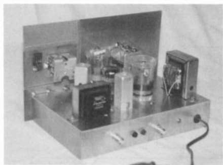
Figure 5. The Multivalue Receiver No. 2, using a Type 14BR11 Compactron in a straight TRF circuit.
