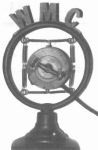
WESTERN ELECTRIC MODEL 387W MICROPHONE – This 1920s double-carbon, spring-type microphone was used in the early days of broadcasting. Radio station WMC celebrated its 75th year on the air in 1998. I worked for the WMC station for 35 years and retired in 1997. (Willis Rudolph – Memphis, TN)
