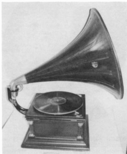
Produced from 1906 to 1915, this Victor 6, with spear-point mahogany horn, was known as "The Gold Tone Model." The unit has an Exhibition reproducer and sold for $5,700.
