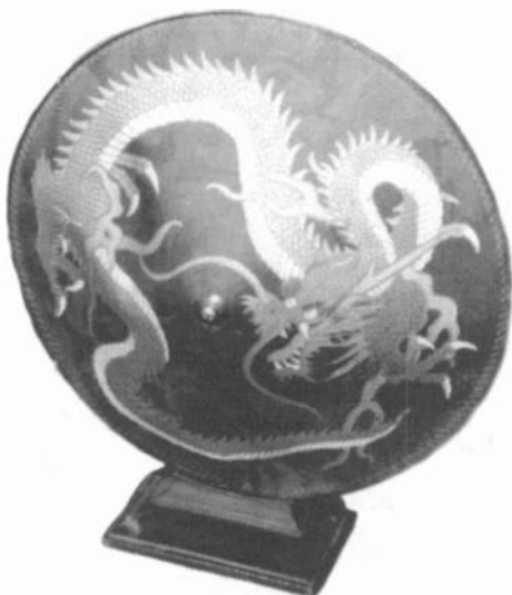
BOSCH AMBORTONE SPEAKER – This dramatic, "dragon motif," cone speaker was manufactured by the American Bosch Magneto Corp. of Springfield, Mass. It measures 18" across the heavily constructed paper cone. (Dave Crocker – Mashpee, MA)
