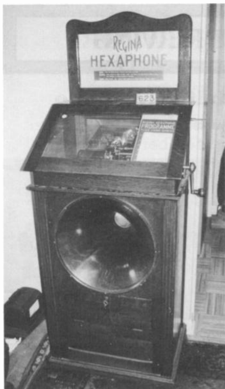
This Regina Hexaphone, an automatic, coin-operated, floor model phonograph, sold for $9,900. Manufactured by the Regina Co. of Rahway, New Jersey from 1908 to 1921, this machine plays cylinder records.
