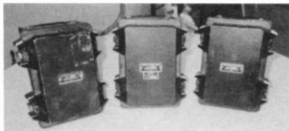
The AN/GRC-109 components with covers on, left to right: power supply, transmitter and receiver. The smaller AC-only power supply is shown at the center.
