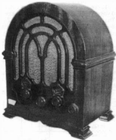
RCA VICTOR MODEL 110 – This 1933 cathedral operates on one each of the following tube types: 58, 2A7, 57, 2A5, and an 80 rectifier. The cabinet is 14 1/4" tall and 11 1/4" wide. (Wally Worth – Wollaston, MA)
