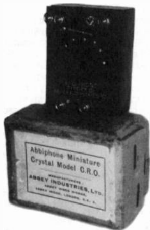
ABBIPHONE MODEL C.R.O. – This miniature catwhisker-type crystal set was made in 1923 by Abbey Industries, Ltd., of London. It measures only 2" x 2 1/2". (Jim Taylor – Boumemouth, England)
