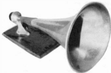
JEROME HORN SPEAKER – This odd-looking speaker was sold by the Jerome Radio Corp. of Chicago in 1922. Incorporating a Baldwin driver at the rear of the spun aluminum horn, it is mounted on a walnut base. This same speaker was sold earlier that year as the Githens speaker by the Auto Parts Mfg. Co. of Detroit. (Dave Crocker – Mashpee, MA)
