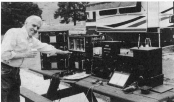
At last year's event, Andy Becker, NONVM, looks over the BC-191 and BC-312 set. This station was operational with dynamotors powered by batteries on the back of the bench.
