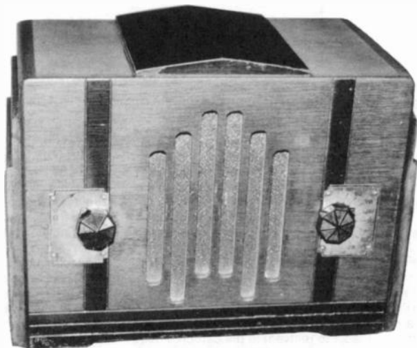
Figure 1. This small 4-tube AC/DC TRF radio of the mid-1930s lacks a manufacturer's name.
