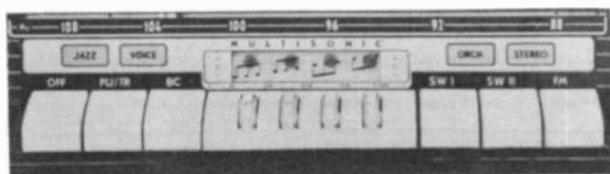
*Figure 2. The piano-style keys control power and function (AM, FM, SW, or phono/tape deck). The thumbwheel controls can adjust bass and treble response.*
