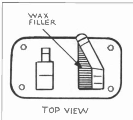
Figure 3. This sketch shows the location of the wax filler that I added to facilitate removal of the pattern from the mold.
