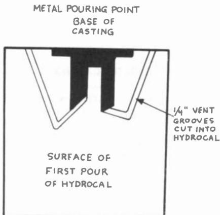
Figure 5. It is necessary to cut paths in the mold to allow air to escape when the molten metal is poured into the mold.
