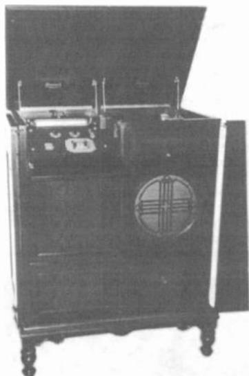
**BRUNSWICK MODEL PR-138C** – This radio-phonograph combination console, called the "Panatropé," was Brunswick's top-of-the-line offering in 1926. The set consists of an RCA Radiola 28 receiver having 8 tubes, a Brunswick 78 rpm phonograph, and a built-in speaker. The AC version sold for \$995, while the DC version sold for \$945. (Donald S. Cockrane – S. San Francisco, CA)
