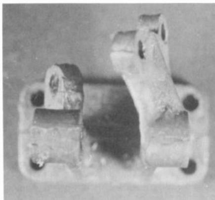
Figure 1. A top view of the original pot metal casting after the dial cord pulleys and shafts were removed. Note the cracked arms and angles of the arms.
