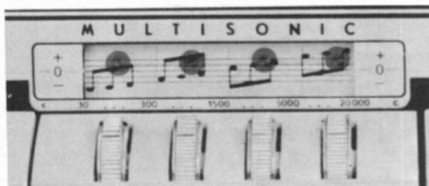
*Figure 3. This detailed view shows the 4 thumbwheel tone controls and their indicators.*
