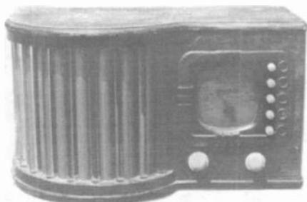
**ZENITH MODEL 5R317** – This is Zenith's "Glass Rod" radio of 1938. Purchased at a second-hand store for \$35, it needed restoration. I replaced three of the glass rods and had repro push buttons installed. It is now in working condition. (James Apthorpe – Leesburg, FL)
