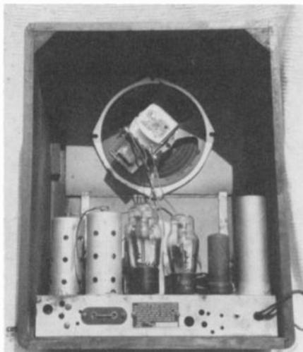
Figure 2. The rear view of the Wilcox-Gay radio showing the chassis, tubes, speaker and, at the bottom, the location of the jumper jack for either radio or phonograph operation.
