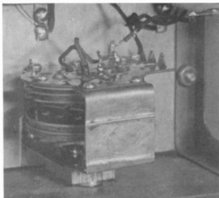
Figure 2. The repaired antenna coil assembly.
