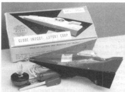
**GLOBE MODEL MG-308** – This highly stylized rocket ship is a germanium crystal radio that tunes with a rod in the ship's nose. It was manufactured by the Globe/Miniman Radio Co. of Japan. (Harry Blesy – Hindsdale, IL)
