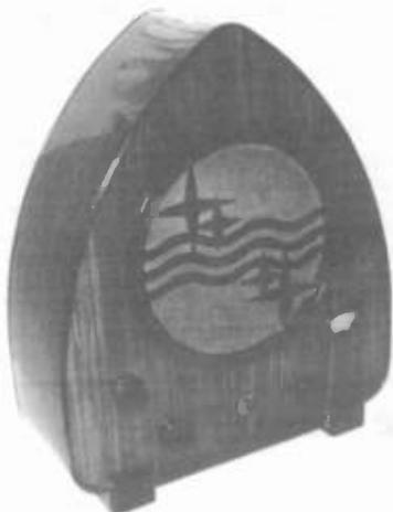
**PHILIPS MODEL 930A** – This 4-tube AC (mains) cathedral receiver was manufactured in London in 1930. The wood-grained cabinet is of Arbolite laminate. (Jim Taylor – Bournemouth, England)
