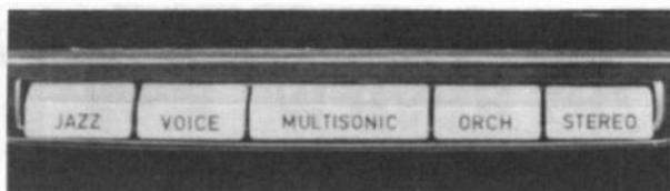
Figure 4. In addition to the variable tone controls shown in Figure 3, the control panel offered the preset tone control positions shown here.
