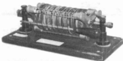
**QUENCHED SPARK GAP, MANUFACTURER UNKNOWN** – This piece of spark equipment sits on a walnut base and has 7 adjustable gaps with glass rod insulators. (Wally Worth – Wollaston, MA)
