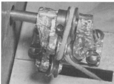
Figure 6. The completed dial-drive assembly installed in the radio.
