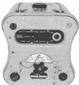
**MAE WEST EMERGENCY RADIO** – Manufactured by Kingston Products Co. of Kokomo, Indiana, this unit was used by downed World War II pilots to call for help. The odd shape was to fit the user's knees while he turned a crank to generate power. (*Clark Trissell – Lincoln, NE*)
