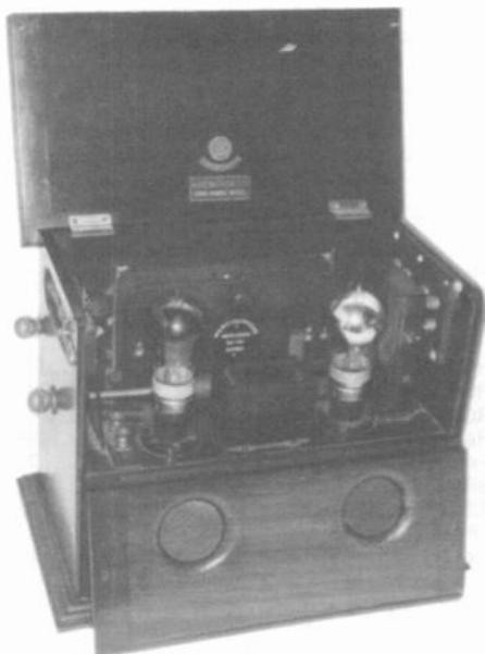
**MARCONIPHONE V2A** – Found in mint condition, this 2-tube, reflex, long-range model receiver was manufactured in 1924. It operates on the 300-390 meter wavelength. (*Jim Taylor – Bourmemouth, England*)
