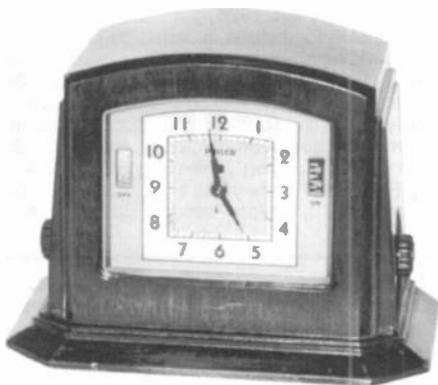
**PHILCO TIMER CLOCK** – This wood-cased timepiece was presumably used to turn on (or off) radios at prescribed times. The knobs on the sides are the familiar Philco rosette type of the early 1930s. (*George E. Hausske – Wheaton, IL*)
