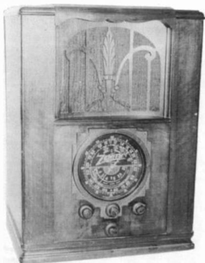
ZENITH MODEL 6S27 – This 6-tube tombstone radio tunes American, foreign, police, amateur and aviation bands. Each dial band is illuminated in a different color. (Clark Trissell – Lincoln, NE)
