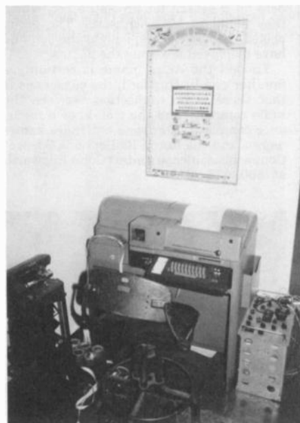
A teletype station. On the wall is a McElroy Mfg. Corp. chart of codes and signals.
