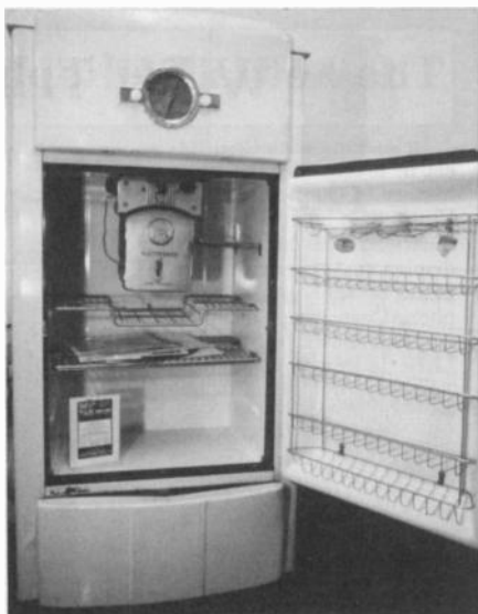
The Crosley refrigerator radio is a refrigerator with a built-in radio, unlike the Westinghouse so-called refrigerator radio which is a small radio resembling a refrigerator.
