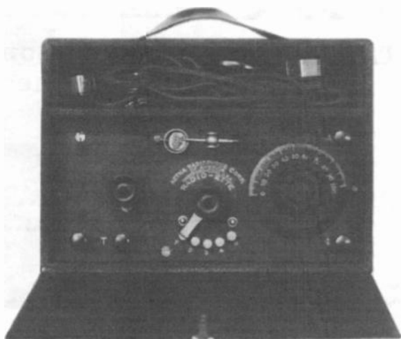
Figure 1. The portable Aetna crystal set with its handle showing and cover down. Seen at the top of the panel is the crystal detector. Under it are the words: "AETNA RADIOPHONE CORP. OF AMERICA, HARTFORD—CONN. U.S.A., RADIO-ETTE." The set has binding posts for antenna, ground, and headphones.
