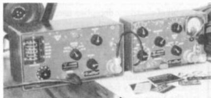
*Bjom Forsberg, SM5UR, set up this operating Swedish paratrooper radio set. Frequency range of the RA-190 is 1.1 to 16 MHz with about 3 watts RF output. A complete set of accessories is in the bag to the right of the set.*
