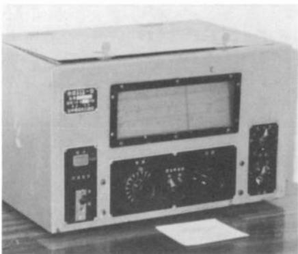
This Japanese "morale receiver" was built in 1943 and has 9 tubes. It operates on the broadcast band and 6-18 MHz. It is owned and operated by Ludwell Sibley, KB2EVN.
