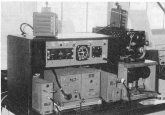
ed points, while the other two are called "Outer" or "Middle" markers (OM/MM). The OM and MM transmitter sets are located on the flight path to the runway for landing purposes. The transmitters are modulated with three different audio tones to activate the lamps.
