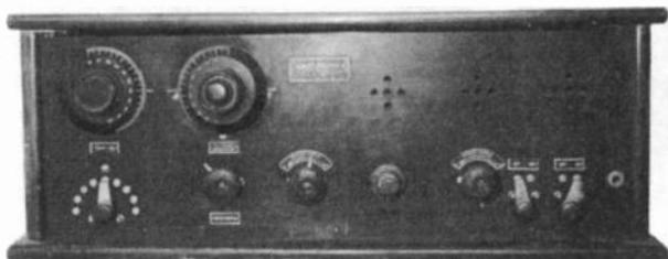
**ARLINGTON RECEIVER** – This 4-tube radio appears to be a super-regenerative tuner followed by the detector stage and two audio stages. It was manufactured by the Wells Manufacturing Company of Fond du Lac, Wisconsin. (*Raymond E. Versaw – Grand Junction, CO*)
