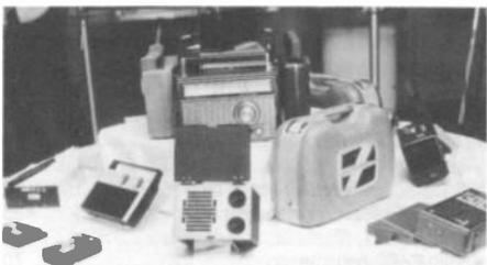
*A variety of portable radios including the 1946 tube-type, suitcase-look-alike "Sporter," right center, and several 1960s transistor radios, left.*
