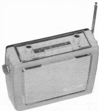
**BLAUPUNKT MULTIBAND TRANSISTOR RECEIVER, MODEL UNKNOWN** - This radio has AM, FM, and two shortwave bands. It has attachments that would allow it to be installed in an automobile but to be easily removed for portable use. (*Joseph G. Jackson - Macon, GA*)
