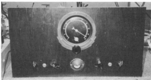
Figure 2. Ed Sheldon's Miller tuner. Note the tuning eye tube at the bottom center. Unlike Dick Parks' tuner that is calibrated in kHz, this tuner has an airplane-type dial calibrated from 0 to 100.
