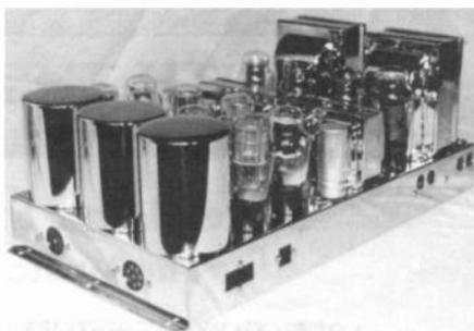
Figure 5. The 12-tube power amplifier chassis.
