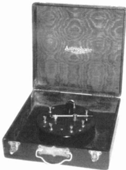
**ASTROPHONE DELUXE CRYSTAL SET** – This unique crystal set was manufactured in the spring of 1923 by Amplifiers Ltd. It is mounted in a black, rexine-covered box with handle, and padded with royal blue watered silk. The set carries the G.P.O. Reg. No. 410. The socket is for an LW plug-in tuning coil for receiving the Paris time signals on 2,600 m. I own two different versions of this novelty set. (Erwin Macho – Vienna, Austria)
