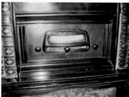
Figure 5. A view of the control panel of the Victor RE-75. The tuning knob is set at its mid-position.
