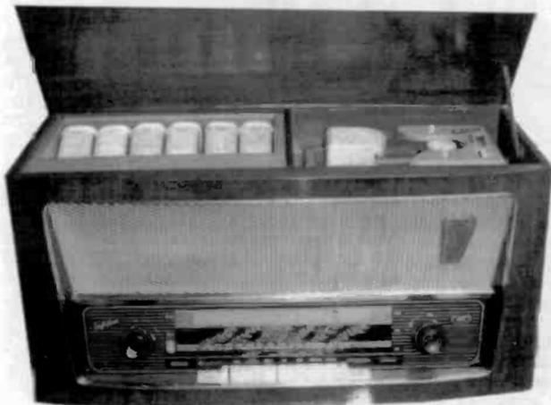
**TEFIFON** - Produced in 1960, this German set was made for only a year and a half. The radio is below, and in the top upper right is a tape unit that plays the large tape cartridges seen stored under the left side of the lid. Each cartridge contains six melodies. (G.W.H. Faassen - Holland)
