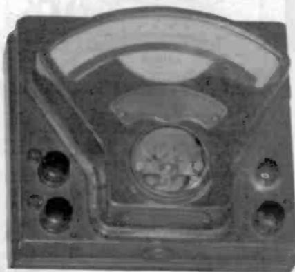
**WESTON MODEL 1DC VOLTMETER** - The cover of this instrument appears to be copper, and it is painted red. The last patent date is July 16, 1901. (Joseph G. Jackson - Macon, GA)
