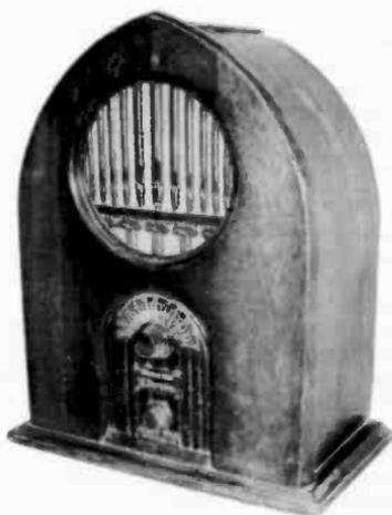
**ZANEY-GILL CLARION**– This 1931 cathedral has a 6-tube chassis. It was manufactured by the Zaney Gill Corporation of Western Avenue in Los Angeles, California. The circular grille trim is cast metal and resembles church organ pipes. The dial escutcheon, which reads "True Vox Clarion, Zaney Gill Corporation," is also cast metal to look like the steps going up to a church. This is truly a "cathedral" radio. (Wally Worth – Wollaston, MA)
