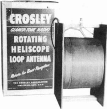
**CROSLLEY ROTATING HELISCOPE ANTENNA** – This loop antenna was recently purchased at a local auction. It has a connection for an outside long-wire antenna with 3 lead wires. It is then rotated for better reception. The box is 7" x 7" x 12". (Everett Hoard – Lehr, ND)
