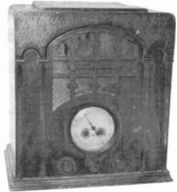
**UNIVERSAL TOMBSTONE, MODEL UNKNOWN** – This 1935 tombstone operates on 32-volt DC battery power. It uses the following tubes: (2) Type 12Z3; (1) Type 12A5; (1) Type 6F7; (1) Type 6D6; and (1) Type 6B7. It tunes both the broadcast and shortwave bands. (Clark Trissell – Lincoln, NE)
