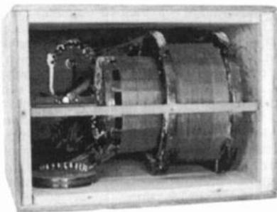
Figure 4. The interior of a Model RLC-5. The RLC-6 contains the same loose coupler.
