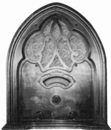
**AUDIOLA MODEL 710** – This 1931, 7-tube cathedral radio uses the following tubes: (2) Type 24; (2) Type 35; (1) Type 27; (1) Type 47; and (1) Type 80. (*Mark Hewitt – Roscoe, IL*)
