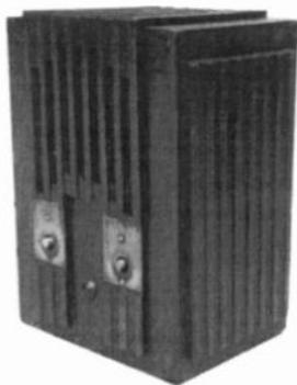
**JEFFERSON MODEL NS40** – Manufactured by the Halson Radio and Television Company, this 1934 TRF midget measures only 10" tall. Its 4-tube complement consists of (1) Type 78, (1) Type 77, (1) Type 43, and (1) Type 25Z5. It has
