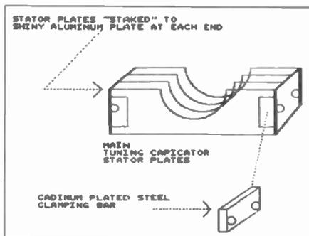
Figure 2. Tuning capacitor stator plate detail.
