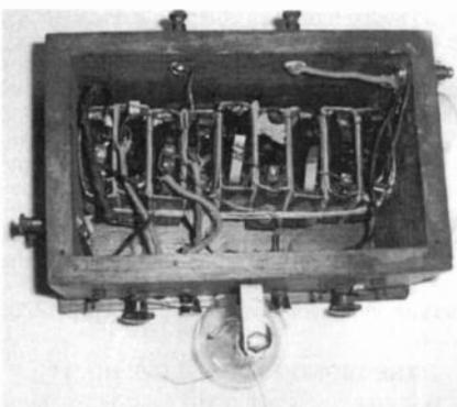
Figure 6. The 9 small batteries of the De Forest JR-4 are exposed because the bottom of the JR-4 was missing.
