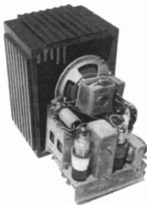
a resistance cord with a red jeweled pilot light. The right metal dial escutcheon is calibrated at 0-100, which is odd for 1934. The 2 knobs and nameplate are missing. (Ralph Jackson – Northboro, MA)
