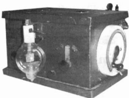
Figure 8. The restored De Forest RJ-4 with the correct rheostat on one end and the spherical Audi-on mounted in the screw type base tube socket.
