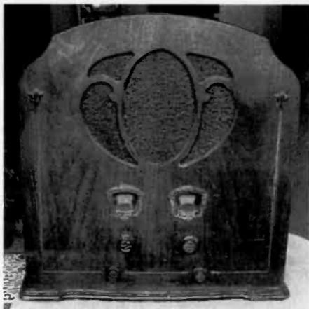
Figure 1. A front view of the 8-tube Kolster Model K-165 with the typical oval pattern grille favored by Kolster.
