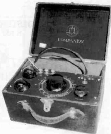
**ICA COMPANION** - This leatherette portable looks as if it should be a battery set, but it is actually an AC portable with two Type 27 Arcturus blue tubes. It measures 11" wide x 6<sup>5</sup>/<sub>16</sub>" tall. (*Wally Worth - Wollaston, MA*)
