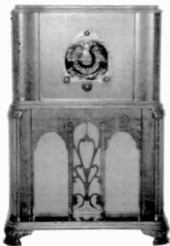
**ZENITH MODEL 15U270** - This 1938 model has Zenith's largest chassis (1501), using 15 tubes with 4 6V6 output tubes yielding 30 watts. The set's features include motorized tuning, a 4-band shutter dial, and a green tuning eye. This was Zenith's only console in 1938 to have two speakers. The price when new was \$225. (*Frank Drost - Woodbury, MN*)
