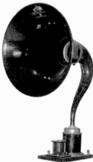
**MAGNAVOX TYPE R2 MODEL B HORN SPEAKER** - This horn speaker came with the Magnavox Type AC-2, Model C amplifier. (*Joseph G. Jackson - Macon, GA*)
