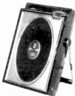
**ZENITH ROYAL 500H** – This early pocket radio uses 8 transistors for reception and 4 Type AA batteries for power. (Clark Trissell – Lincoln, NE)
