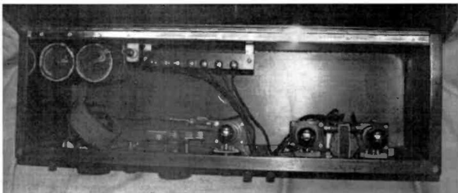
Figure 3. A view of the internal workings of the Haynes-Griffin Dx receiver showing the layout of the components.
