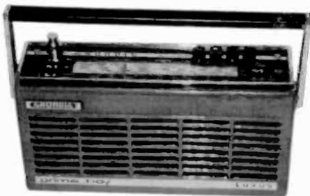
**GRUNDIG PRIMA-BOY LUX** - This is a fine transistor portable of the late 1960s. It has no AC power cord and operates only on batteries. It receives the following European ranges: UKW, KW, MW, and 49m. (Erwin Macho - Vienna, Austria)
