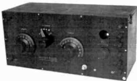
Figure 2. Closeup of the 1-tube receiver section. (From the John V. Terrey collection.)
