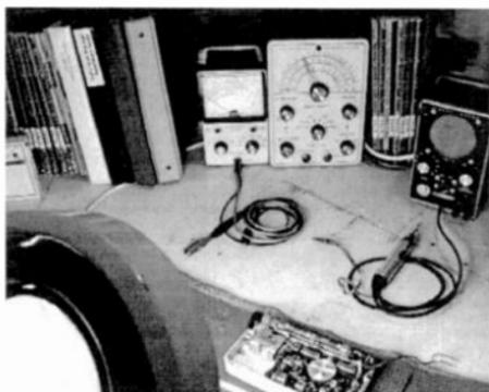
Figure 2. The equipment required for electronic testing of transistor radios need not be elaborate. These inexpensive Heathkit units will do the job.
