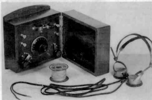
**HOME-BREW CRYSTAL SET** – I designed and built this catwhisker type crystal set using old antique parts. Housed in an old meter case, it works very well with a pair of Western Electric headphones. (*Joseph Wood – Hodgkins, IL*)
