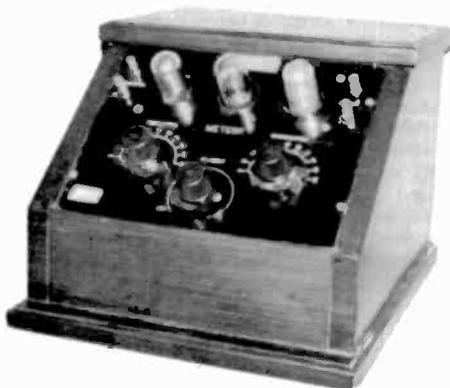
**ECHOPHONE MODEL A** – This set is a 3-tube regenerative receiver with a detector and two stages of transformer-coupled audio. It may have originally used Type 12 tubes, as it has a large battery compartment, big enough for a couple of No. 6 dry cells, plus a couple of B batteries and a C cell. It was found with Type 201-A tubes in all three sockets. (George Hausske – Wheaton, IL)
