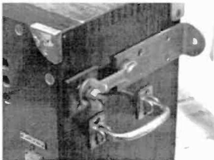
Figure 8. Detail showing the heavy brass construction of the latch, bracket and handle.
