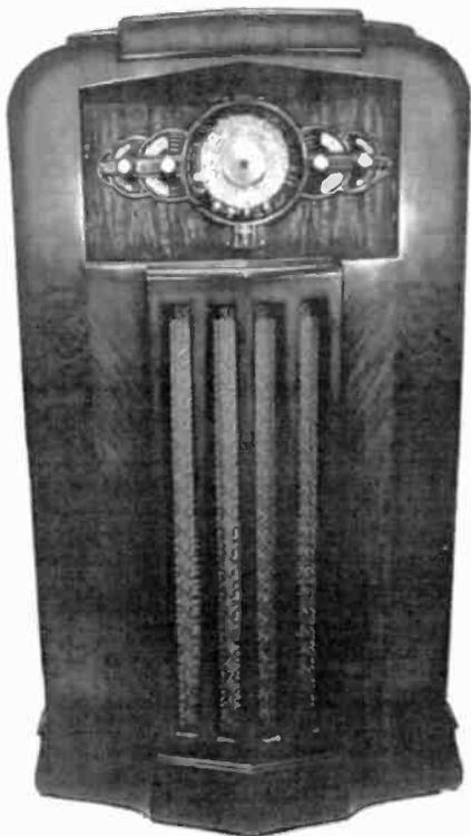
Figure 2. This Midwest Model 18-37 is an example of a radio cabinet in which the grille cloth must fit the angular shape of the cabinet's grille.
