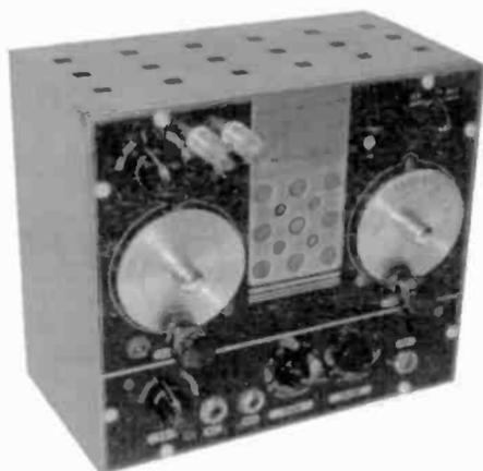
**ABBOTT INSTRUMENT MODEL TR-4** – This ultra shortwave receiver/transmitter was manufactured in the U.S.A. in the 1940s. (*Jim Taylor – Bournemouth, England*)
