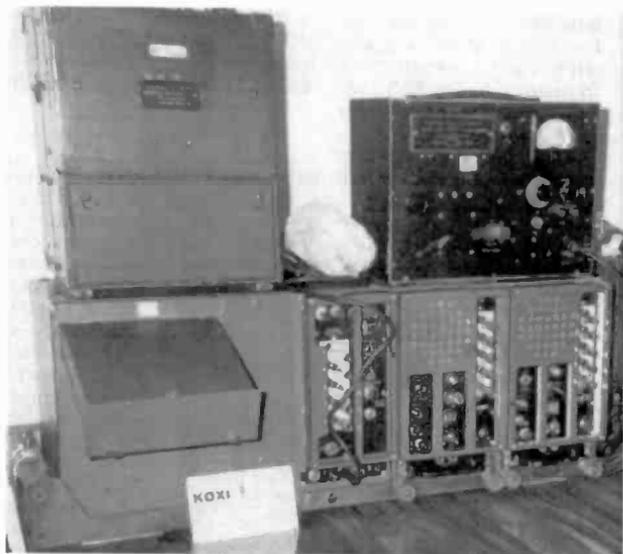
*Two pieces of test equipment are sitting on top of this SCR-608 VHF FM set. The transmitters and receivers operated in the band from 20 to 40 MHz and were installed in a number of army tanks. The open drawer at the left contains extra crystals for frequency changes. Phil Epstein brought the set from Minneapolis for display.*
