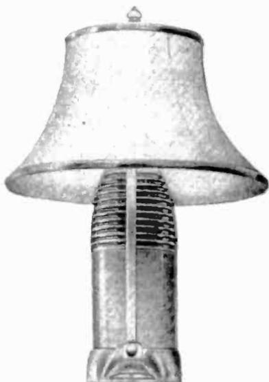
**MITCHELL LUMITONE** – This ceramic lamp has a radio inside its hollow frame. Tuning is done by a horizontal thumbwheel at the base. At the top of the lamp is an opal plastic reflector bowl. The shade is made of celanese taffeta with gold piping. It stands  $21\frac{1}{8}$ ” tall and the shade diameter is 16”. (Fielding L. Grigsby – Ft. Smith, AR)
