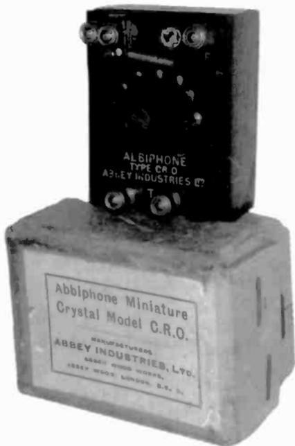
**ABBIPHONE MODEL C.R.O.** – Manufactured in 1924 by Abbey Industries, Ltd., of London, this tiny crystal set measures only  $1\frac{1}{2}$ ” x  $2\frac{1}{2}$ ” at the base. (Jim Taylor – Bournemouth, England)
