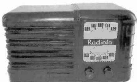
**RADIOLA MODEL 500** – Manufactured by RCA Victor, this circa 1941 midget radio has a 5-tube chassis in a walnut Bakelite cabinet. The tube complement is Types 12SA7, 12SK7, 12SQ7, 35Z5, and 50L6. (Jim Ligouri – Atkinson, NH)
