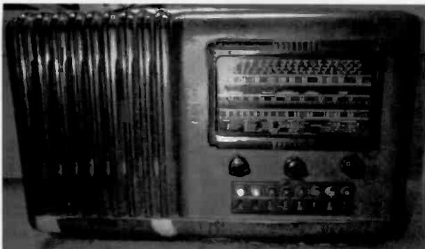
Figure 1. The 8-tube, 3-band radio in its "as found" state. Note the missing veneer on the lower edge of the cabinet.
