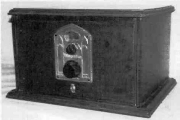
*Figure 1. A front view of the restored Wurlitzer "Navaho" Model. The large knob is the tuning control and the small knob controls volume. The toggle switch below the escutcheon is the on-off switch.*
