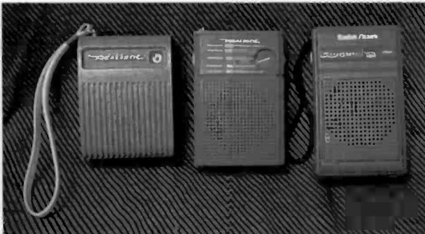
Figure 1. The Flavoradios were produced in three basic case styles. Left to right, the Models 12-166/12-166A, 12-201, and 12-201A.
