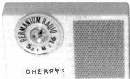
**CHERRY CRYSTAL RADIO** – This tiny, plastic, germanium crystal radio was manufactured in the 1960s. Notice the small compass built into the center of the tuning dial. (*Erwin Macho – Vienna, Austria*)
