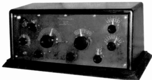
**ZENITH 1R** – This 1-tube receiver was manufactured by the Chicago Radio Laboratory in 1922. It has Serial Number 2369 and is licensed under the Armstrong U.S. patent of October 6, 1914. The front panel is made of hard rubber with a red coloration. The rear has a pull-down door to access the chassis. (*Wally Worth – Wollaston, MA*)
