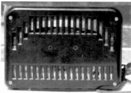
Figure 2. While many AC/DC radios from the 1940s used cardboard back covers, the Lyric used a Bakelite cover.
