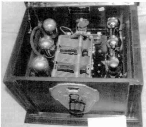
Figure 4. Except for the tube types, the Cherokee's chassis layout seems identical to the Wurlitzer.
