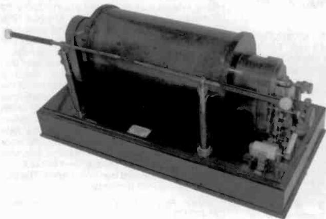
**MARCONI SPARK COIL** – This very heavy piece of wireless equipment was manufactured by the Marconi Wireless Telegraph Company, Ltd., London. The nameplate states that it is "No. 404." (*Jim Taylor – Bournemouth, England*)
