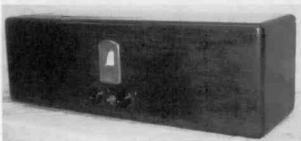
Figure 6. This 9-tube AC-operated Wurlitzer is housed in a cabinet that resembles a Radiola 17.
