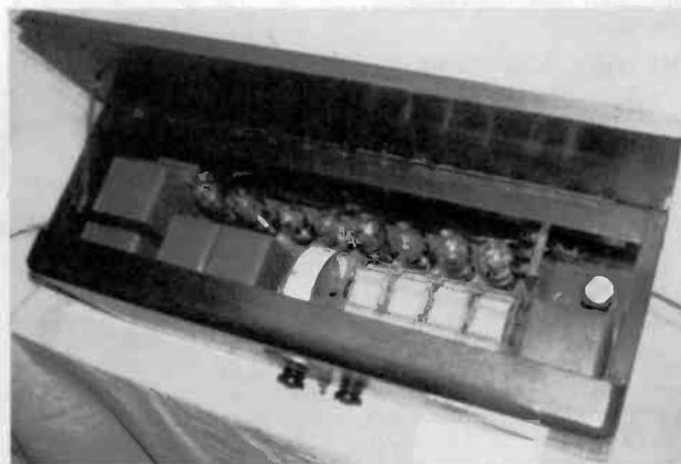
Figure 7. A top view of the 9-tube Wurlitzer shows a chassis layout that looks like a Radiola 17.
